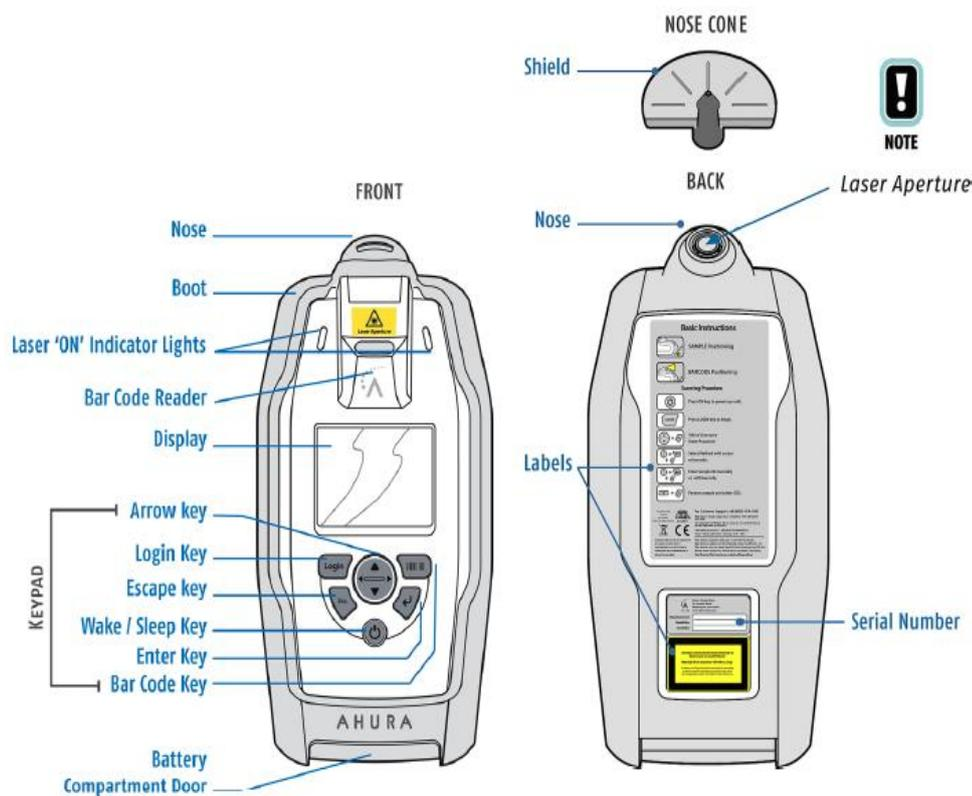
Figure 2.2: TruScan Portable Raman Spectrometer. (TruScan user manual, 2010)
