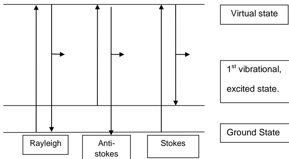
Figure 1.8. The three different types of scattering. (Adapted from Bell, 2006)
