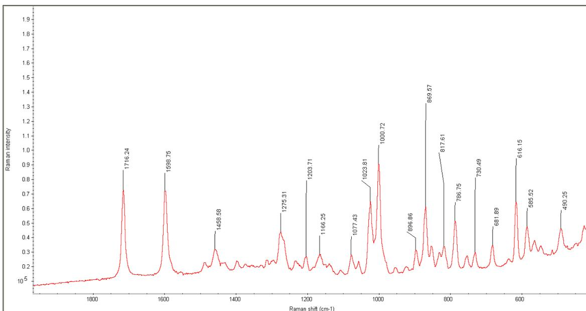
Figure 3.1: Cocaine Hydrochloride reference spectra.
