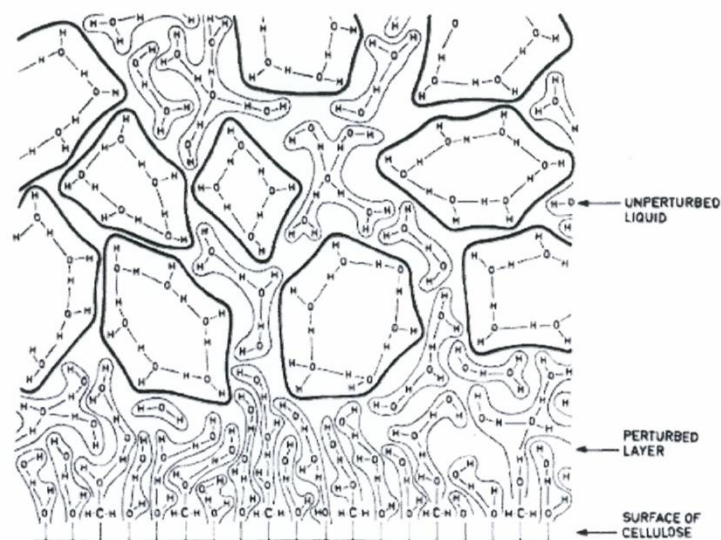
Figure 2.8 Goring's model of fibre water interaction (Goring 1978).
