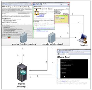
Figure 1. Architecture of the virtual router environment
