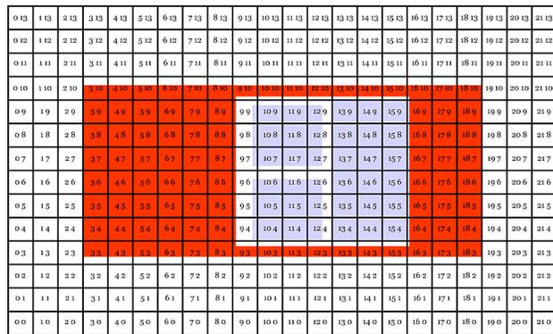
Figure 1: Simplified aerial view of car with grid, red = bodywork, blue = seats
