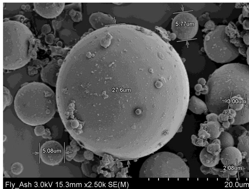
**Fig. 4.12** SEM image of PFA specimen
