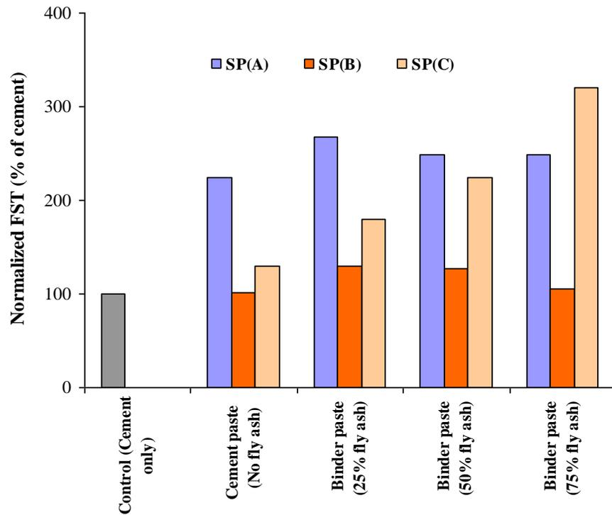
**Fig. 4.19** FST of mixes at different level of PFA and SP with respect to standard mix
