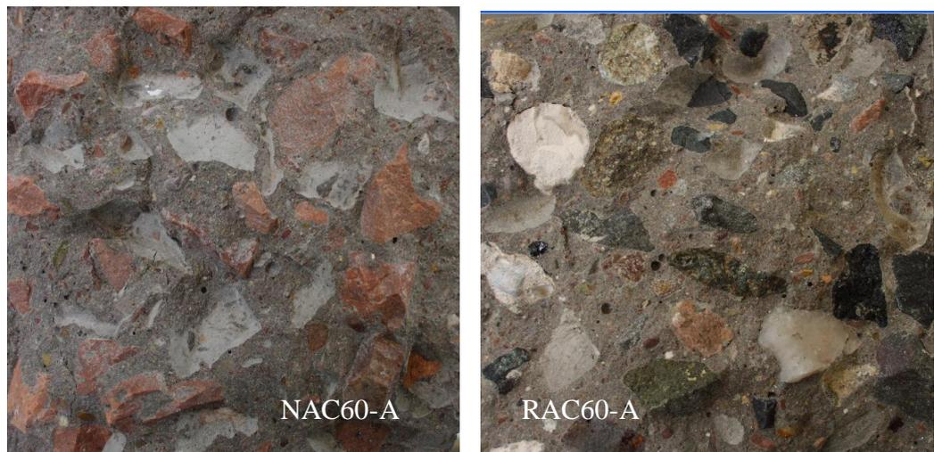
**Fig. 5.10** Fracture surface of samples NAC 60-A and RAC 60-A
