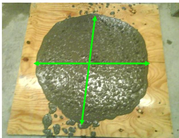
**Fig. 8.9** Measuring flow diameter of a successful SCC mix
