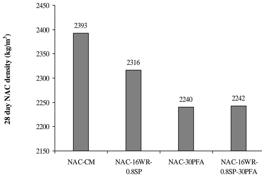
**Fig. 7.12** Influence of PFA cement replacement on the bulk density of NAC concrete
