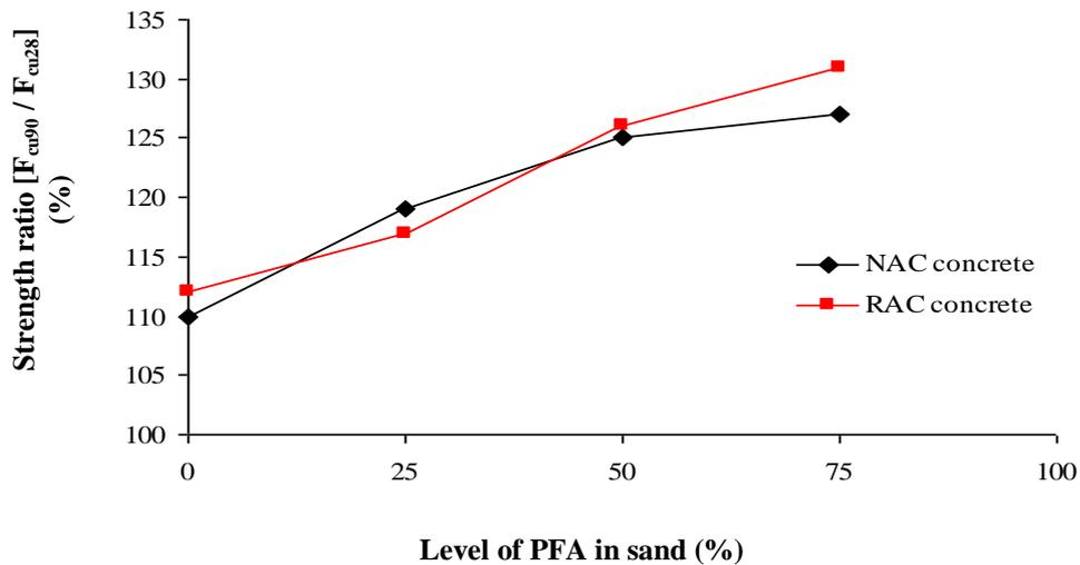
**Fig. 6.2** Influence of PFA level in sand on compressive strength ratio
