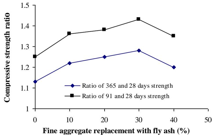
**Fig. 3.4** Compressive strength ratio *versus* fine aggregate replacement with fly ash (after Rafat 2003a)
