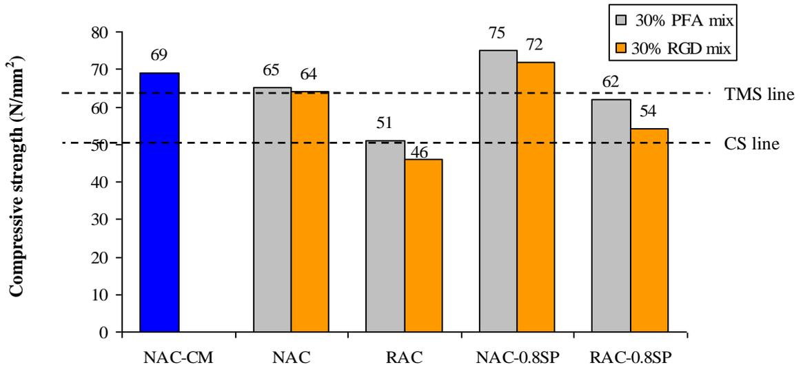
**Fig. 7.29** Comparison of 28 day compressive strength of mixes with PFA and RGD
