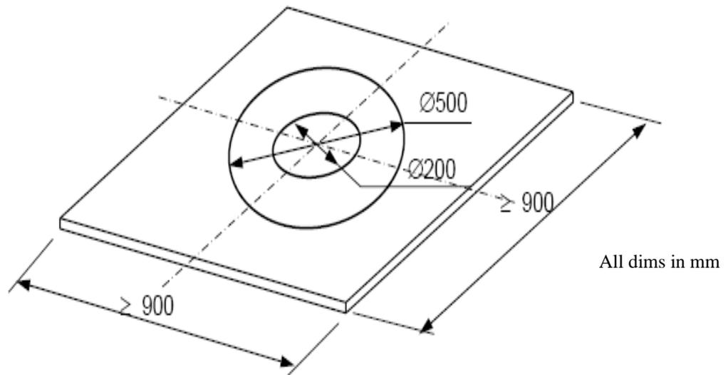
**Fig. 8.1** Dimensions and marking of the base plate (EFNARC 2005)
