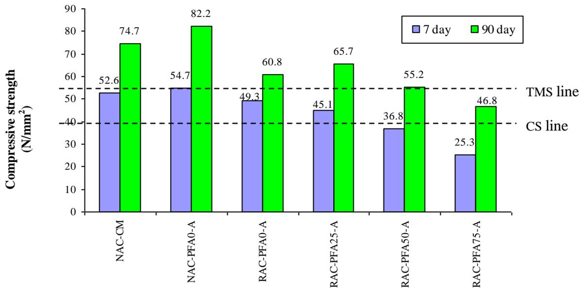
**Fig. 6.3** Compressive strength of RAC concrete produced with different PFA levels and SP type A at early (7 days) and later age (90 days)
