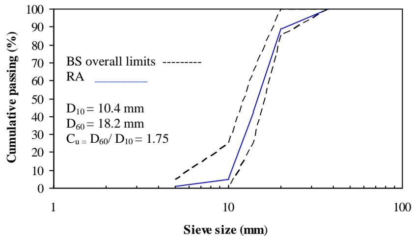
**Fig. 4.3** Grading of recycled coarse aggregate
