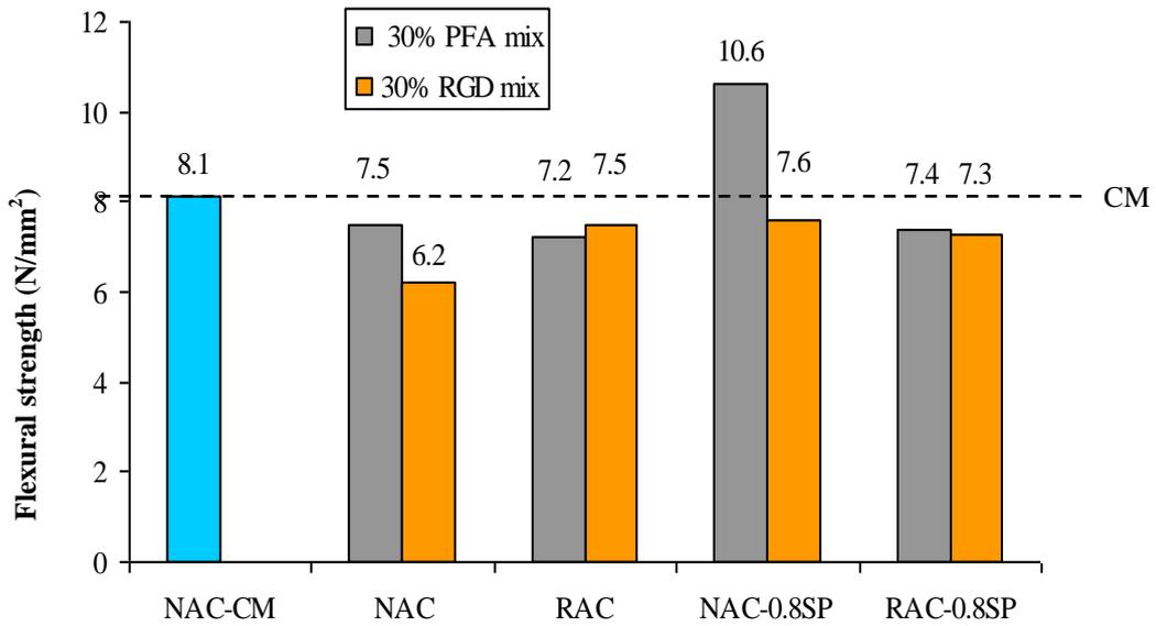
**Fig. 7.31** Comparison of flexural strength of mixes with PFA and RGD and the 28 day control mix
