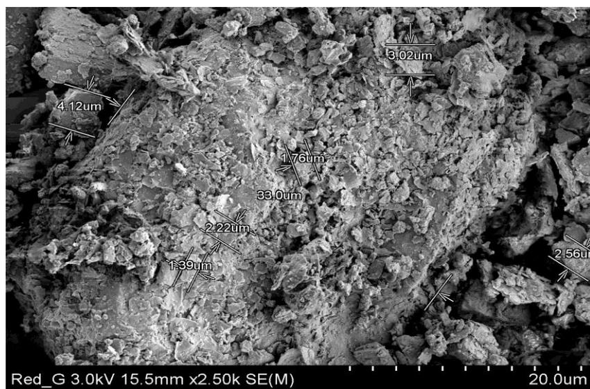
**Fig. 4.14** SEM image of RGD specimen
