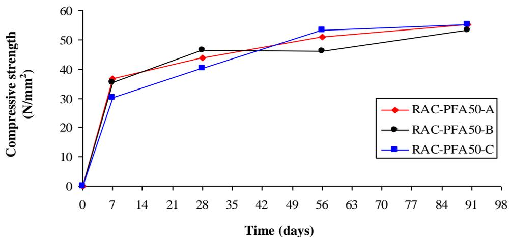
**Fig. 6.4** Compressive strength of RAC concretes produced with 50% PFA and different SP types compared with the control mix
