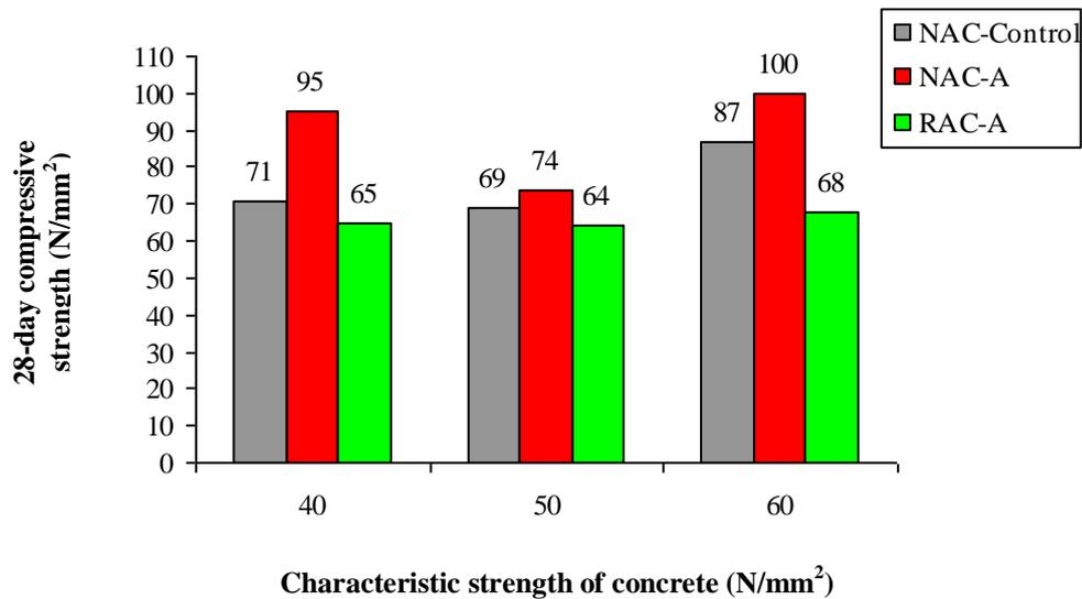
**Fig. 5.6** Compressive strength for NAC and RAC mixes produced with SP type A
