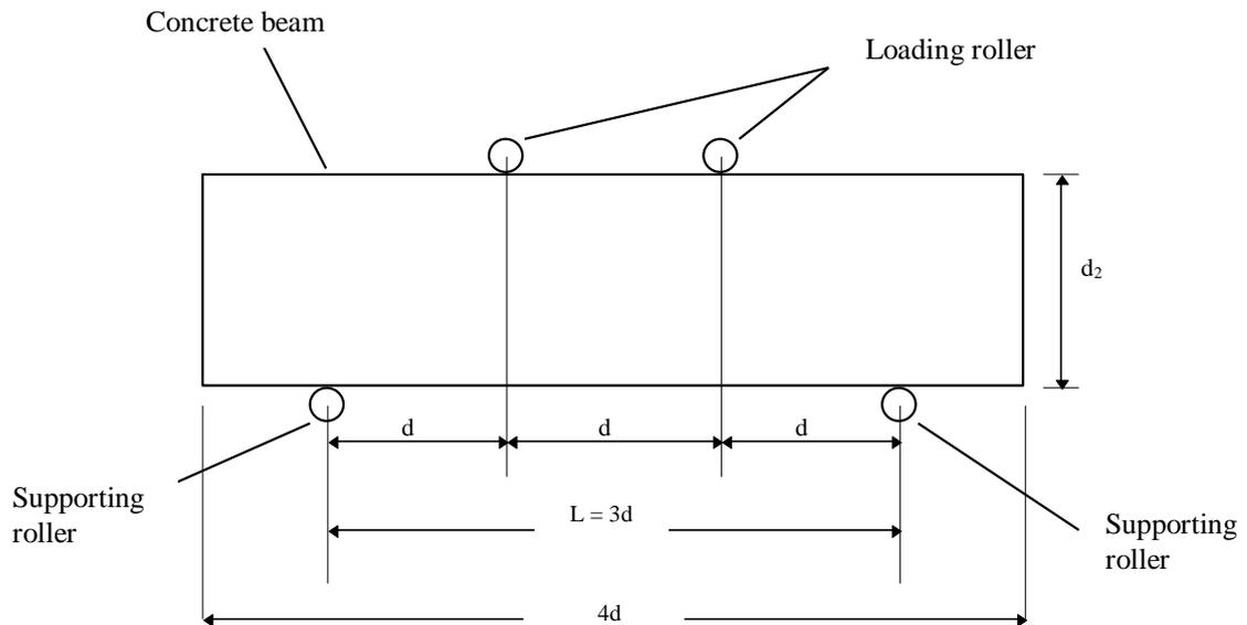
**Fig. 5.3** Arrangement of loading test piece (two point loading)
