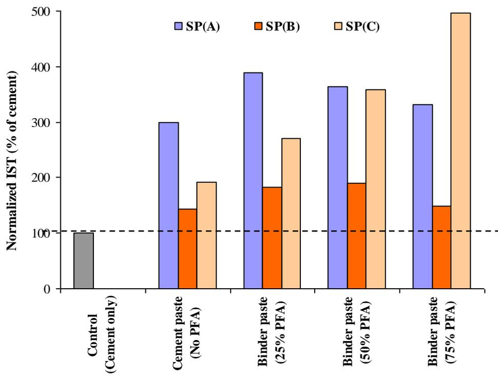
**Fig. 4.18** IST of mixes at different level of PFA and SP with respect to standard mix
