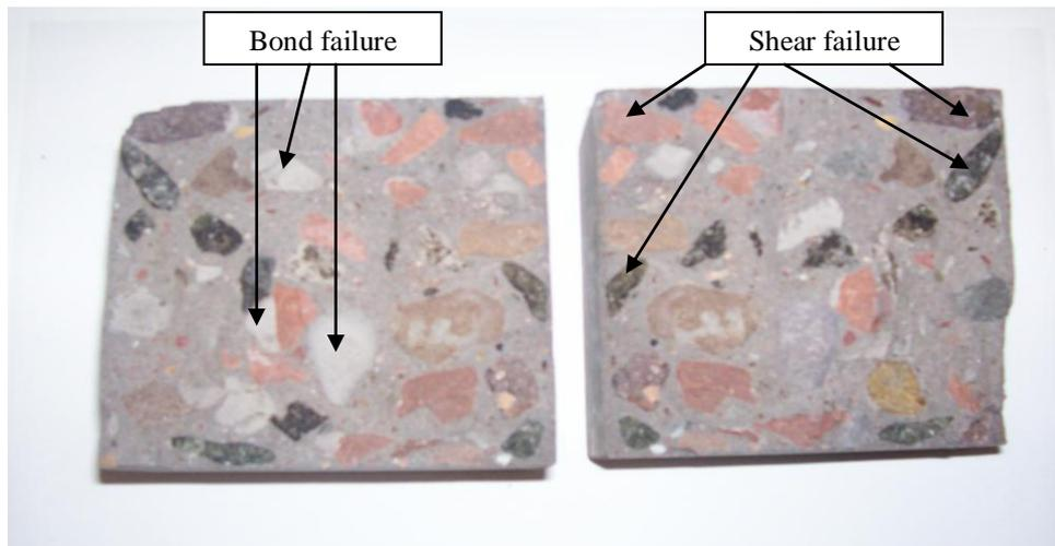
**Fig. 5.11** Fracture surface of NA50-RA50 (blended aggregate concrete)
