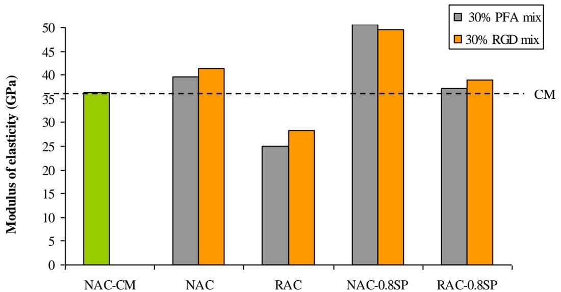
**Fig. 7.32** Comparison of modulus of elasticity of mixes with PFA and RGD and the 28 day control mix
