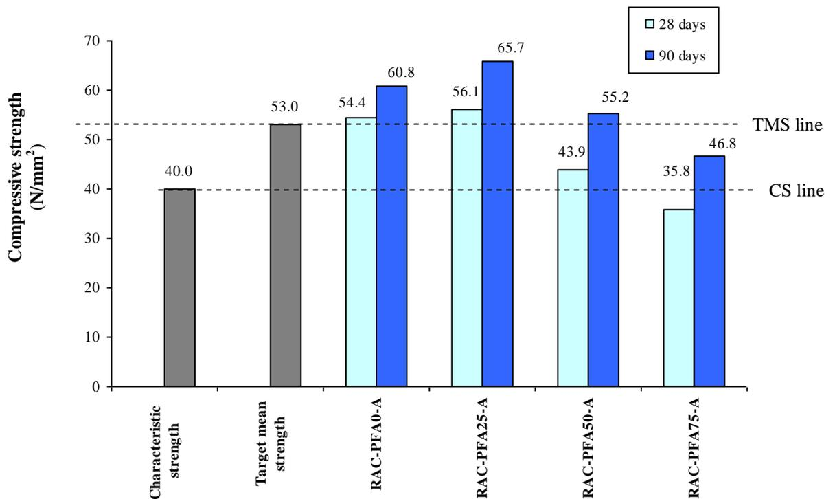
**Fig. 6.7** Compressive strength of RAC concrete as compared with mix design values
