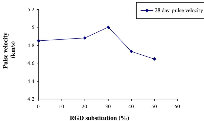
**Fig. 7.22** Variation of pulse velocity of concrete with the level of RGD cement substitution
