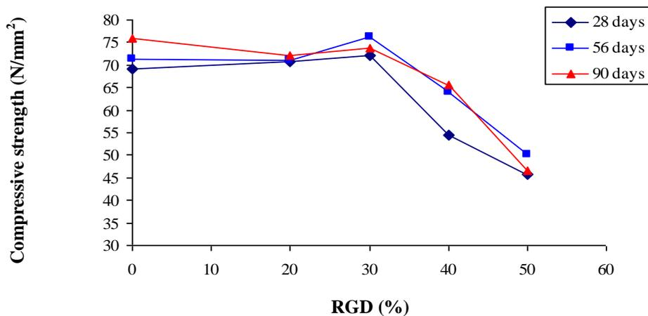
**Fig. 7.19** Compressive strength of different RGD concretes at different ages
