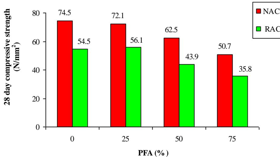
**Fig. 6.5** The 28 day compressive strengths of concrete produced with different PFA contents (SP A used)
