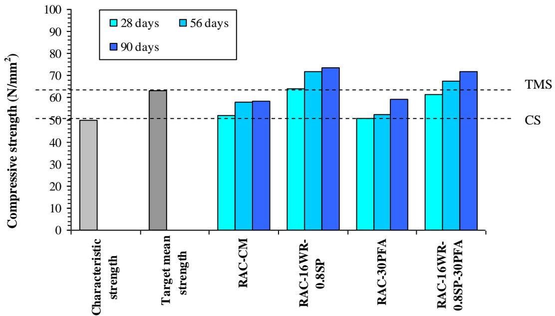
**Fig. 7.3** Compressive strength of RAC mixes with PFA at different ages compared to control mixes
