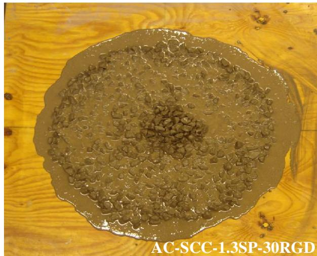
**Fig. 8.8** Failed mixes due to segregation between coarse aggregate and cement paste although the mix passed the flow test
