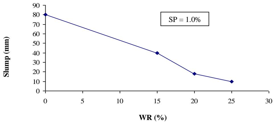
**Fig. 4.30** Relationship between slump and WR for 1.0% SP
