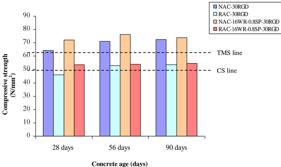
**Fig. 7.25** Comparison of compressive strength of mixes with RGD at different ages
