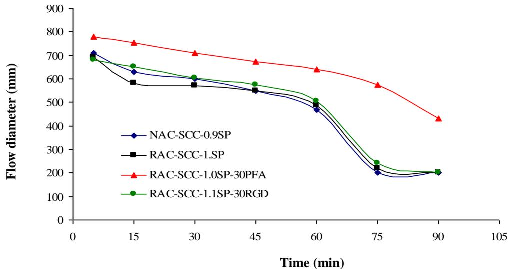
**Fig. 8.14** Flow diameter against time
