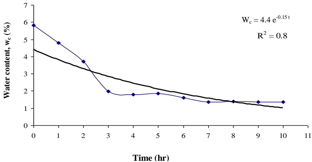
**Fig. 4.9** Drying of RA over time
