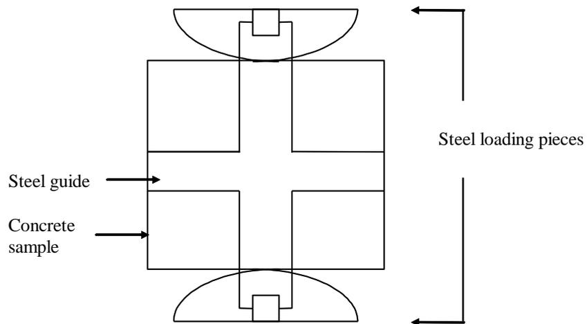
**Fig. 5.1** Loading arrangement for tensile splitting strength
