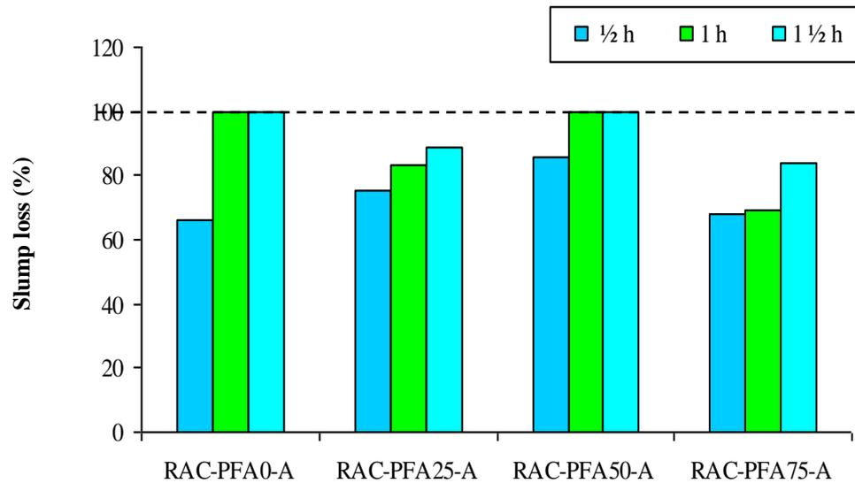
**Fig. 4.23** Influence of PFA content on the rate of slump loss of RAC made with SP A
