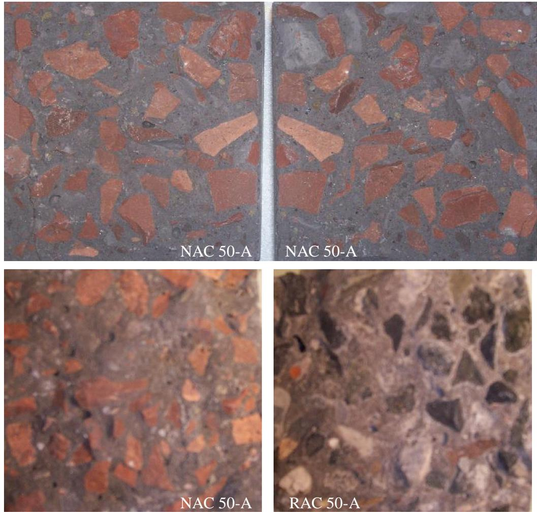
**Fig. 5.9** Fracture surface of samples NAC 50-A and RAC 50-A
