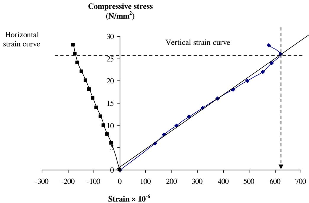
**Fig. 7.27** Stress-strain curve for RGD specimen (NAC-30RGD)
