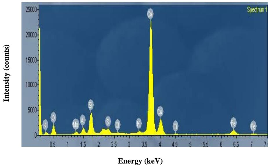
**Fig. 4.11** Spectrum of the energy of characteristic X-rays emitted from the cement specimen
