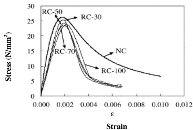
**Fig. 3.1** Typical stress-strain ( $\sigma$ - $\epsilon$ ) curves of RAC (Jianzhuang *et al.* 2005)
