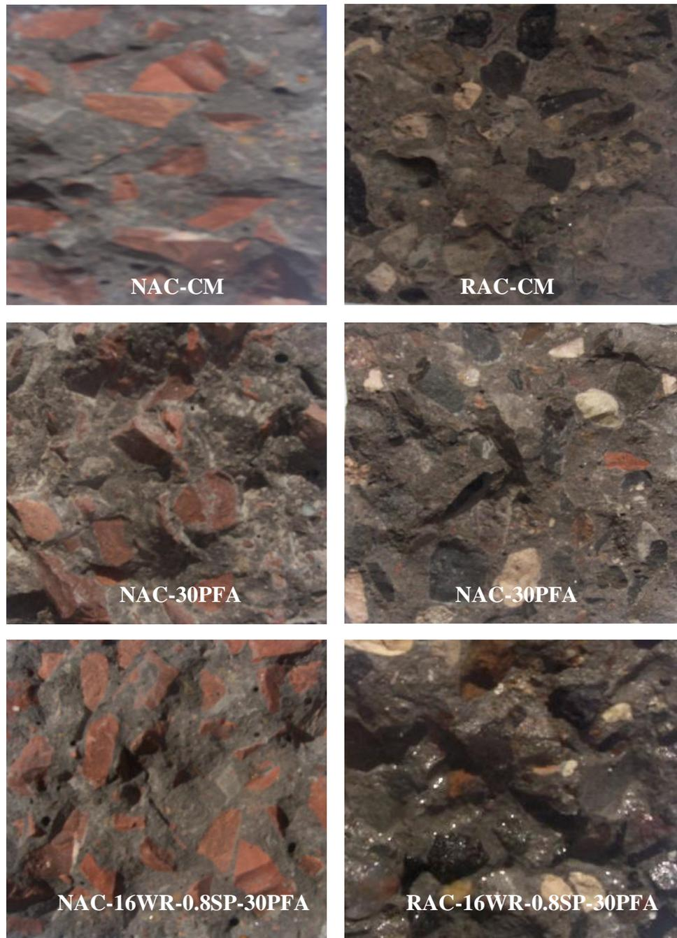
**Fig. 7.7** Fracture surfaces of concrete samples
