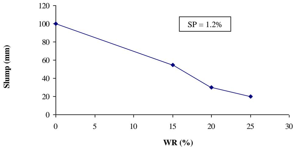
**Fig. 4.31** Relationship between slump and WR for 1.2% SP
