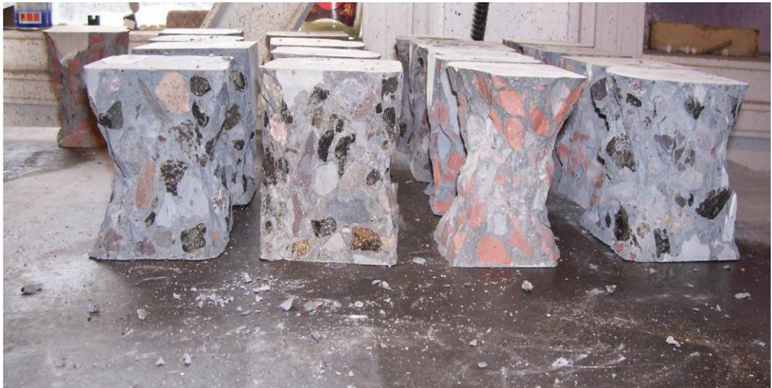
**Fig. 6.8** The shape of crushed RAC and NAC concrete samples
