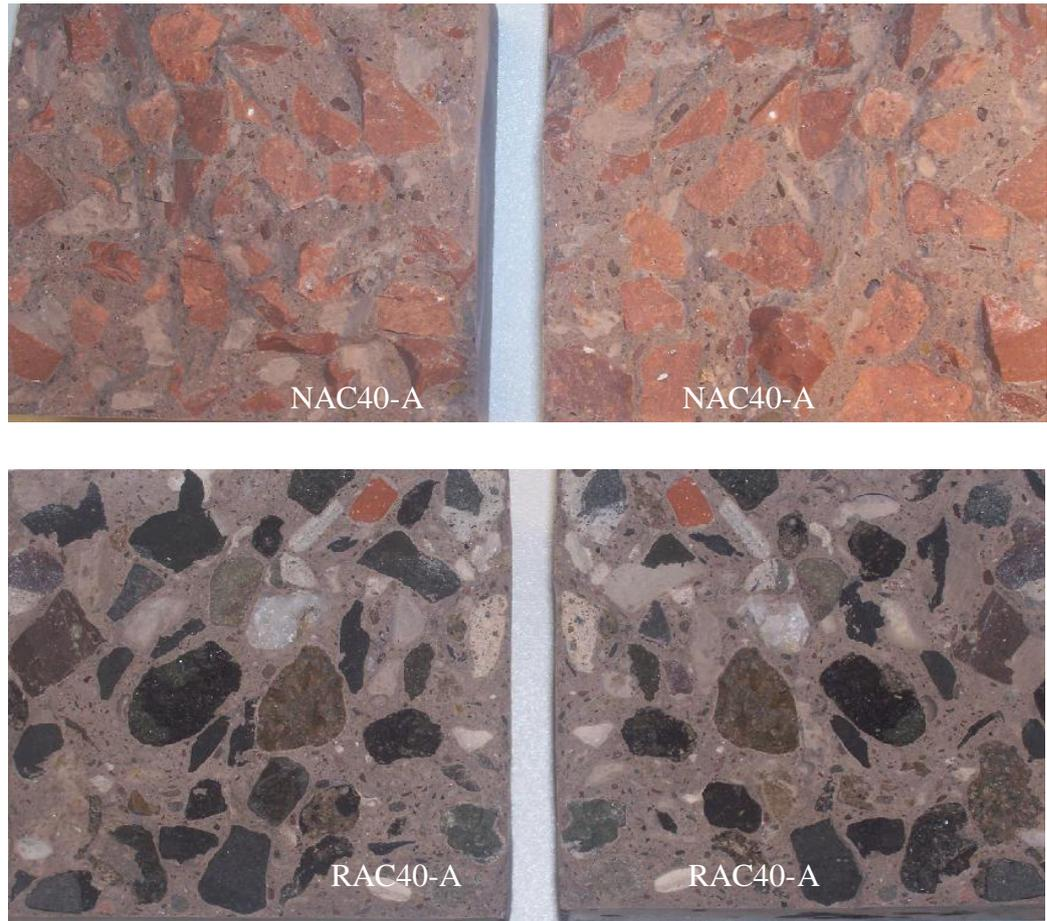
**Fig. 5.8** Fracture surface of samples NAC 40-A and RAC 40-A
