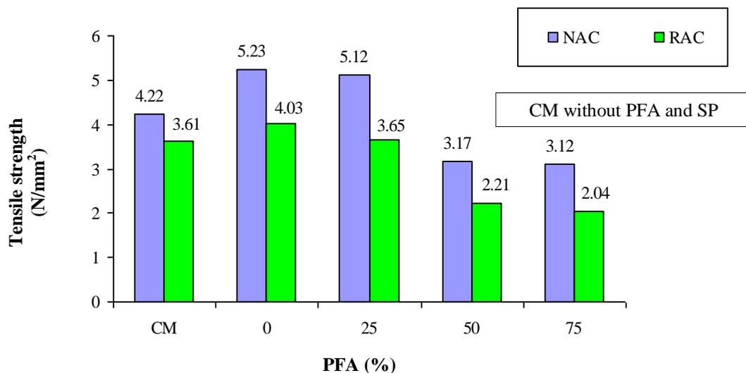
**Fig. 6.9** The 28 day tensile strengths produced with different levels of PFA and SP A
