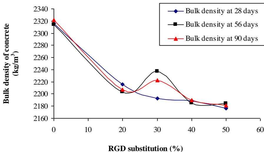
**Fig. 7.21** Variation of concrete bulk density with binder RGD content
