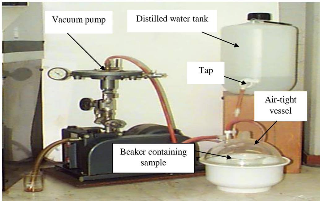
**Fig. 4.7** Porosity testing apparatus
