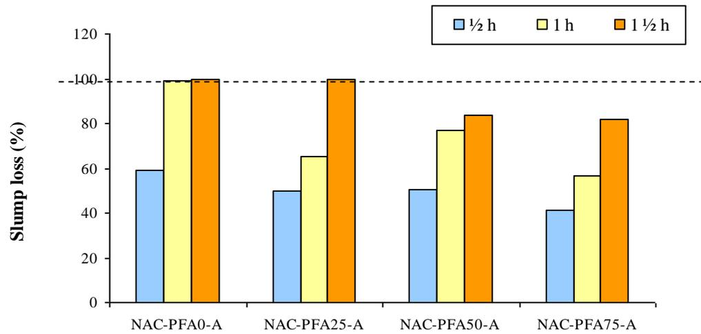
**Fig. 4.22** Influence of PFA content on the rate of slump loss of NAC made with SP A
