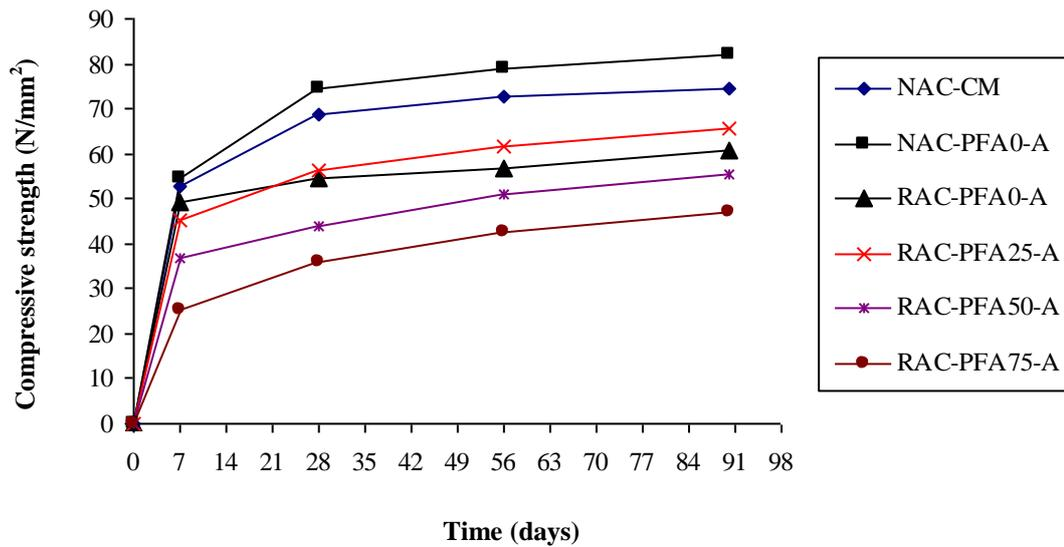
**Fig. 6.1a** Development of compressive strength of RAC with PFA replacing fine aggregate at different levels (SP type A used) compared to the control mix
