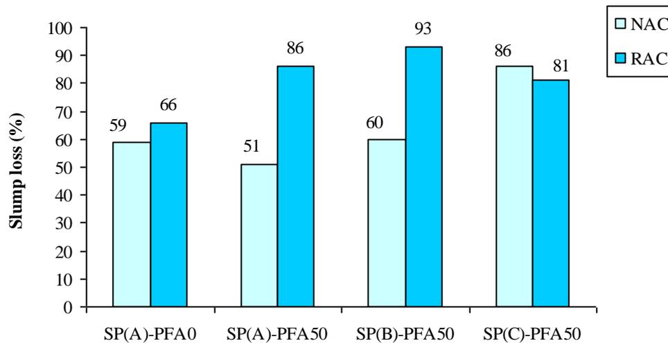
**Fig. 4.21** Influence of SP type on slump loss at 30 minutes for mixes with 50% PFA replacement
