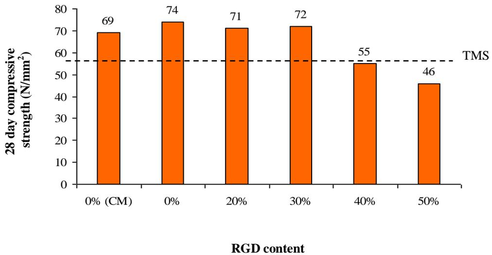
**Fig. 7.18** Compressive strength of different RGD concretes at 28 days
