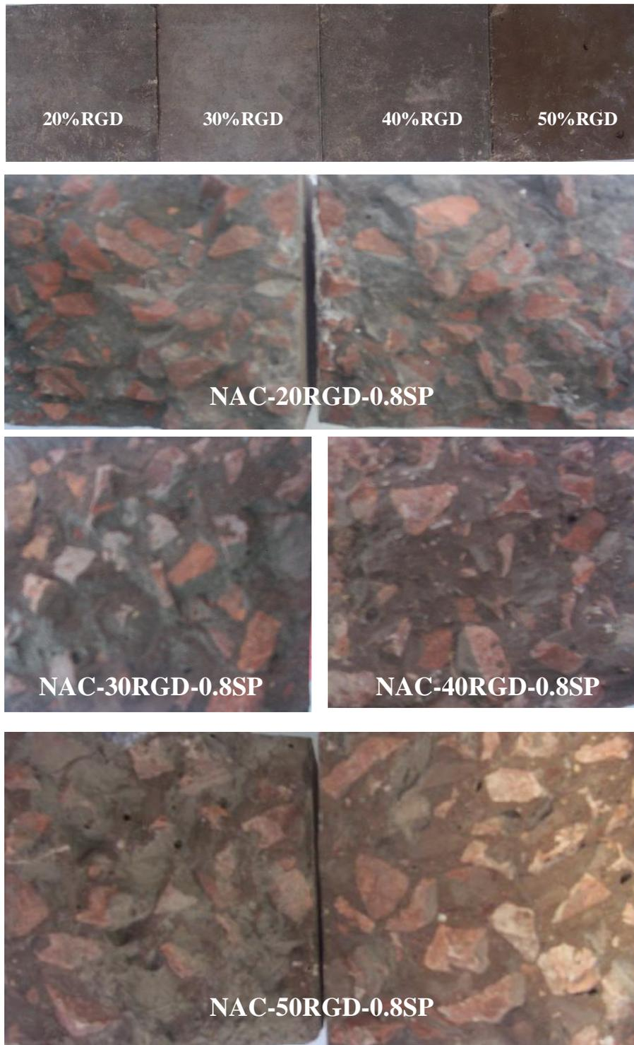
**Fig. 7.17** Concrete cubes and fracture surfaces with different RGD content
