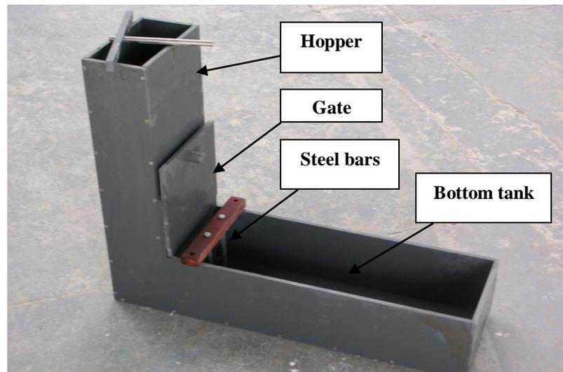
**Fig. 8.4** L-box apparatus
