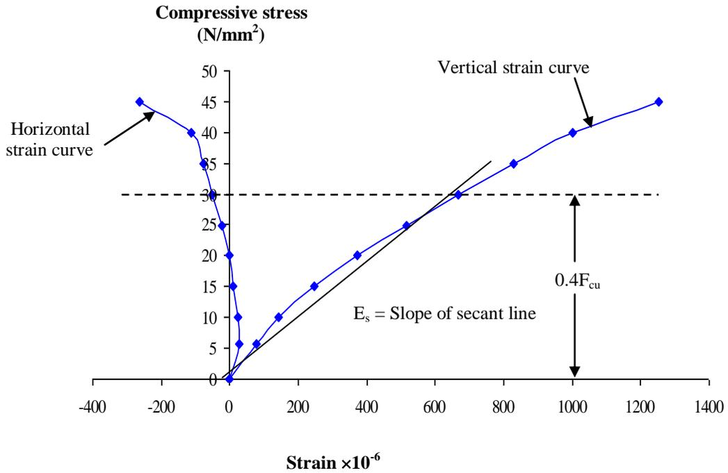
**Fig. 7.10** Typical stress-strain curve for NAC specimen (NAC-CM)
