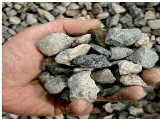
**Fig. 2.5** The variability in shape, texture, and origin (seen simply by colour) of the RA
