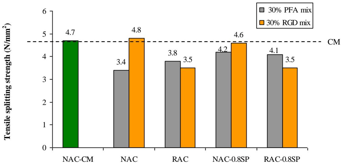
**Fig. 7.30** Comparison of tensile splitting strength of mixes with PFA and RGD and the 28 day control mix
