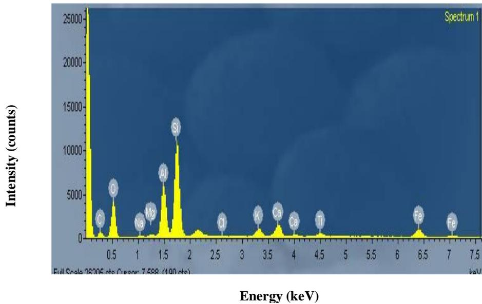
**Fig. 4.13** Spectrum of the energy of characteristic X-rays emitted from the PFA specimen
