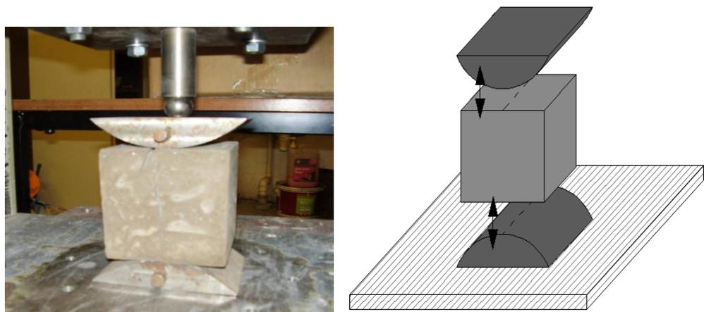
**Fig. 5.2** Loading of a cube for tensile splitting testing (L) and cube alignment (R)
