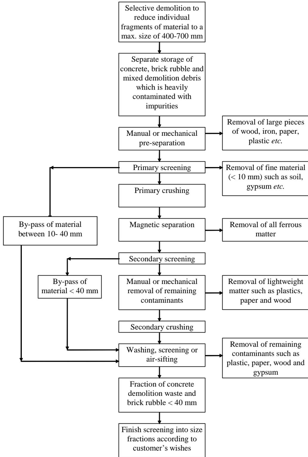
**Fig. 2.11** Processing of demolition wastes (Devenny 1999)
