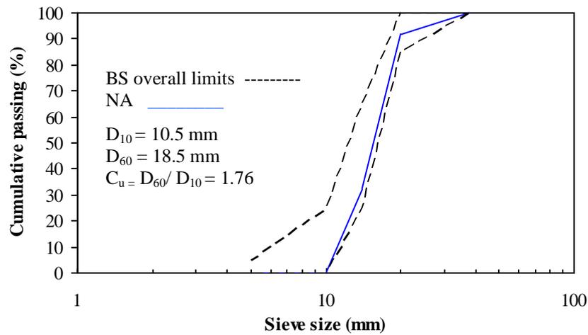
**Fig. 4.2** Grading of natural coarse granite aggregate
