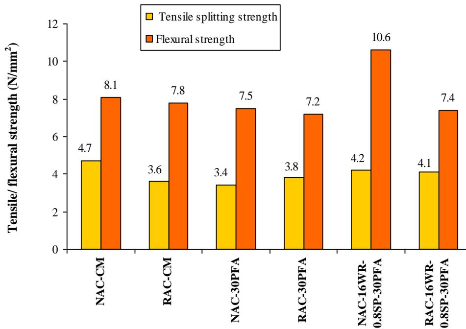
**Fig. 7.6** Tensile splitting and flexural strength of mixes (NAC and RAC) with PFA compared to control mixes
