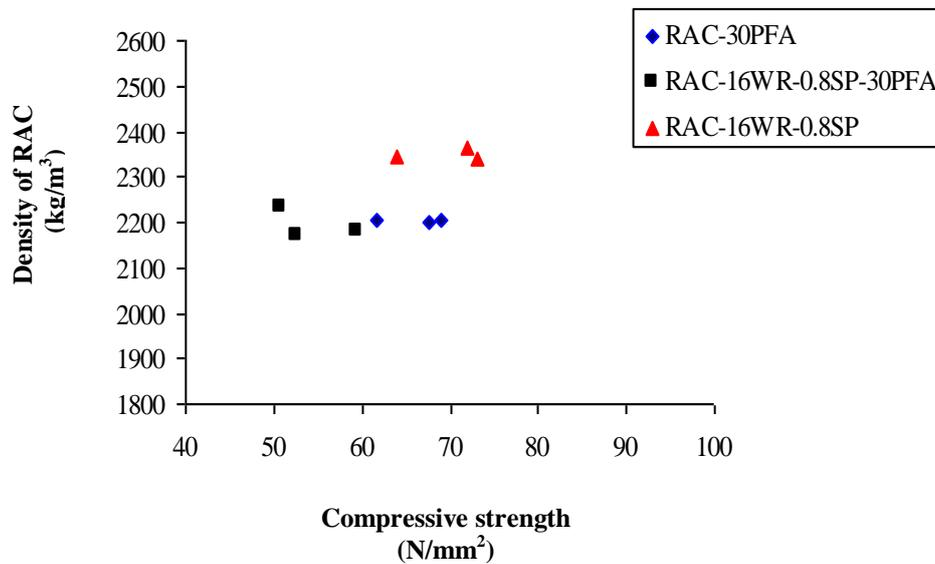
**Fig. 7.14** Density of RAC mixes with admixtures at different ages against the corresponding compressive strength.
