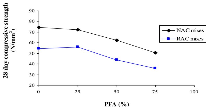
**Fig. 6.6** Influence of PFA content on the compressive strength of concrete
