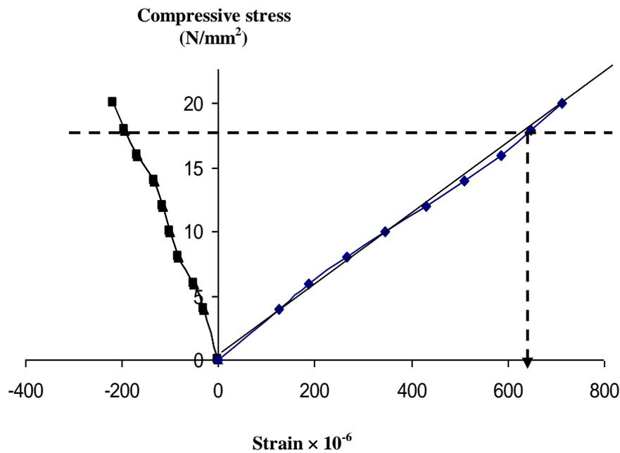
**Fig. 7.28** Stress-strain curve for RGD specimen (RAC-30RGD)
