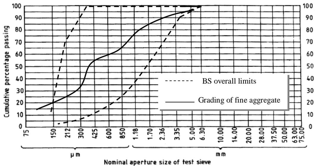
**Fig. 4.4** Grading of fine concrete aggregate
