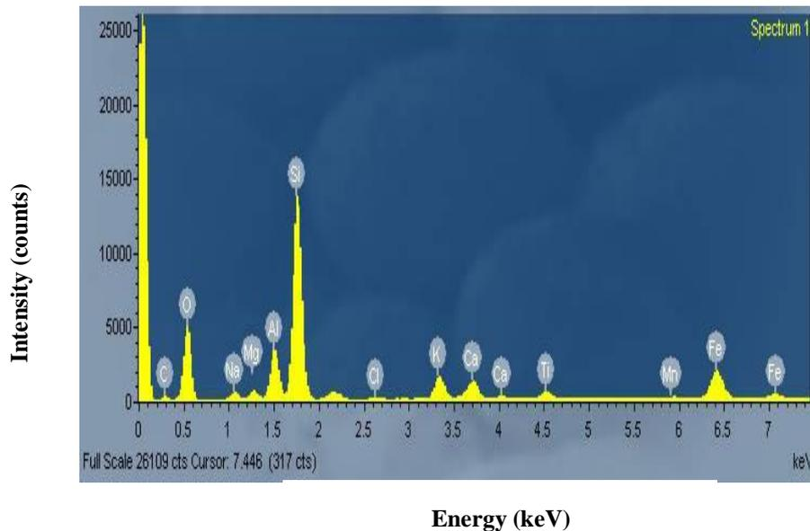
**Fig. 4.15** Spectrum of the energy of characteristic X-rays emitted from the RGD specimen
