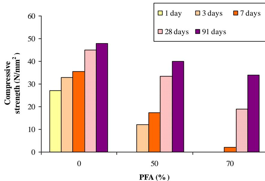
**Fig. 3.2** Variation of compressive strength with the level of PFA and age (Naik *et al.* 1994)
