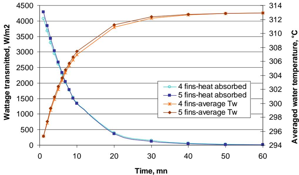
Figure 7: Heat transfer and water temperature profiles in the ICS-SWH with time
