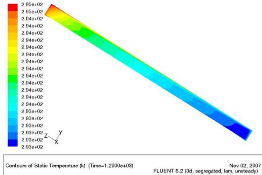
Figure 6: Longitudinal water temperature stratification - 5 fins, side view, after 20mn
