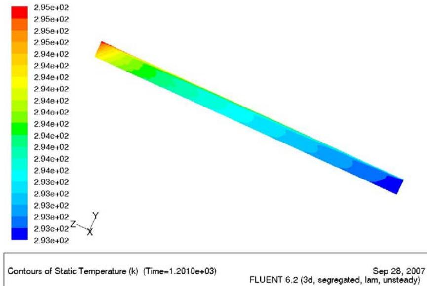
**Figure 4: Longitudinal water temperature stratification – 4 fins, side view, after 20mn**
