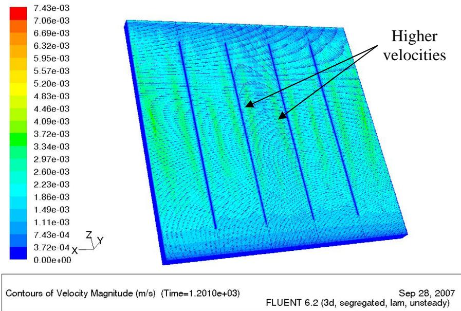
**Figure 3: Velocity profile – 4 fins, top view, after 20 mn**
