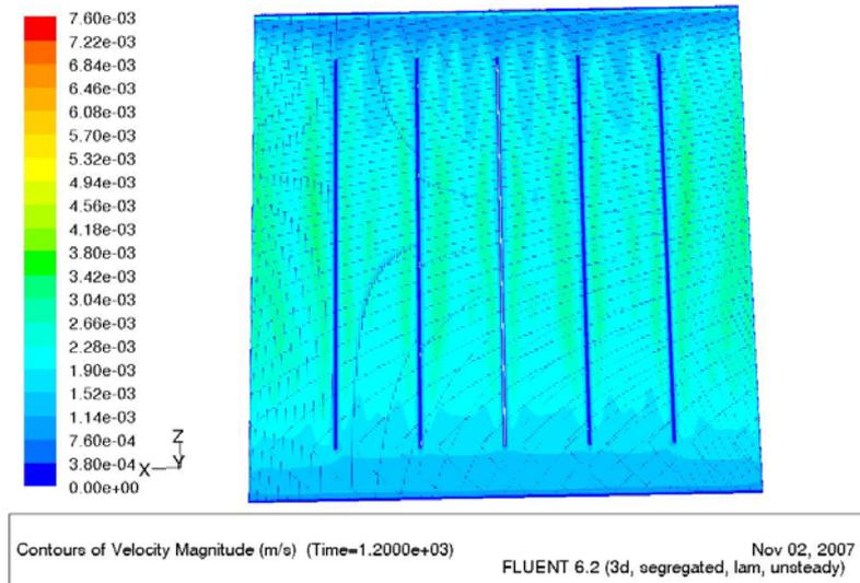
Figure 5: Velocity profile – 5 fins, top view, after 20 mn
