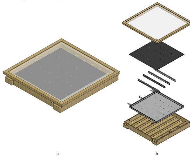
Figure 1: Solar water heater assembly, a: Plain view, b: Explode view
