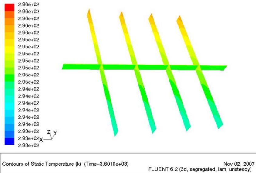
**Figure 2: Temperature stratification of fins and middle line of water collector**
