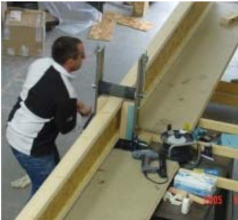
b) Passing the beam through Roller press
