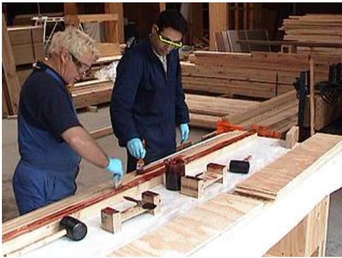
(a) Applying the glue to the grooving area
