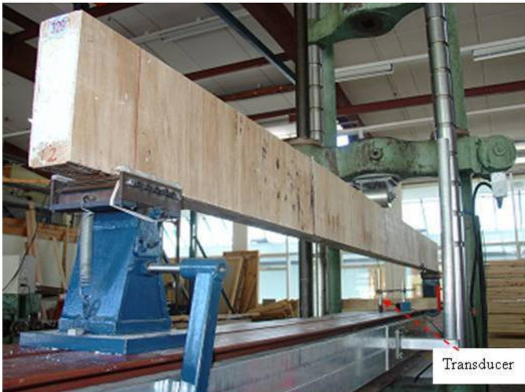
**Figure 4.8 (b) Three points load test rig to measure load-deflection of filled boxed I-Beam over a 4.5m span**
