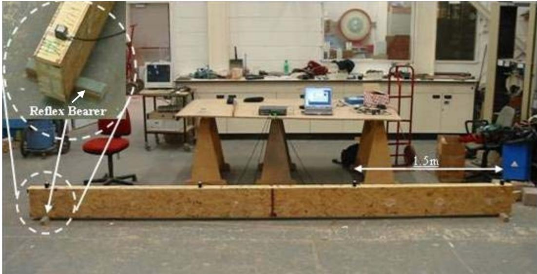
c) Typical dynamic test set up
