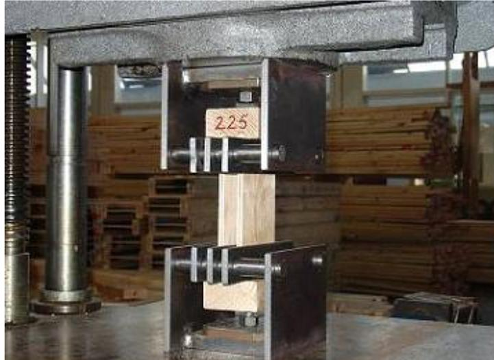
(b) Testing the pulling resistance of a Double I-Beam
