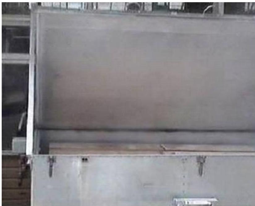
**Figure 4.14 Exposing the beams to steam and at 100 °C**
