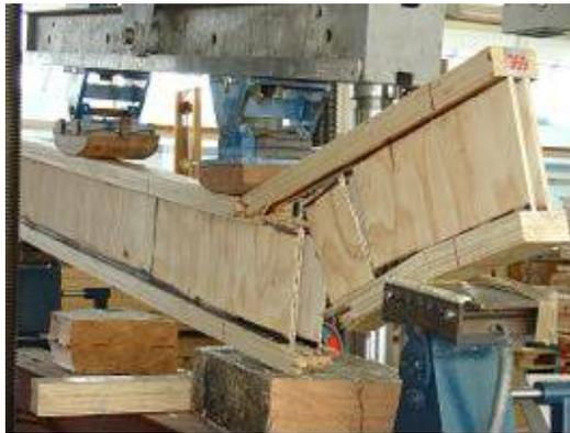
(a) A short span double I-beam
