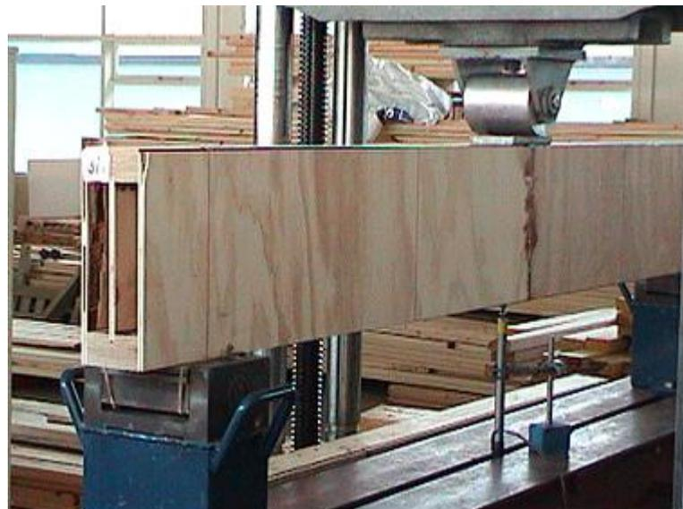
c) Testing Boxed I-beam under three point bending
