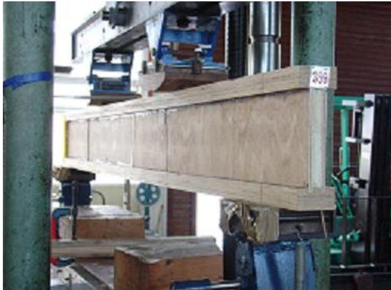
b) Filled LVL double I-beam under four-point-bending
