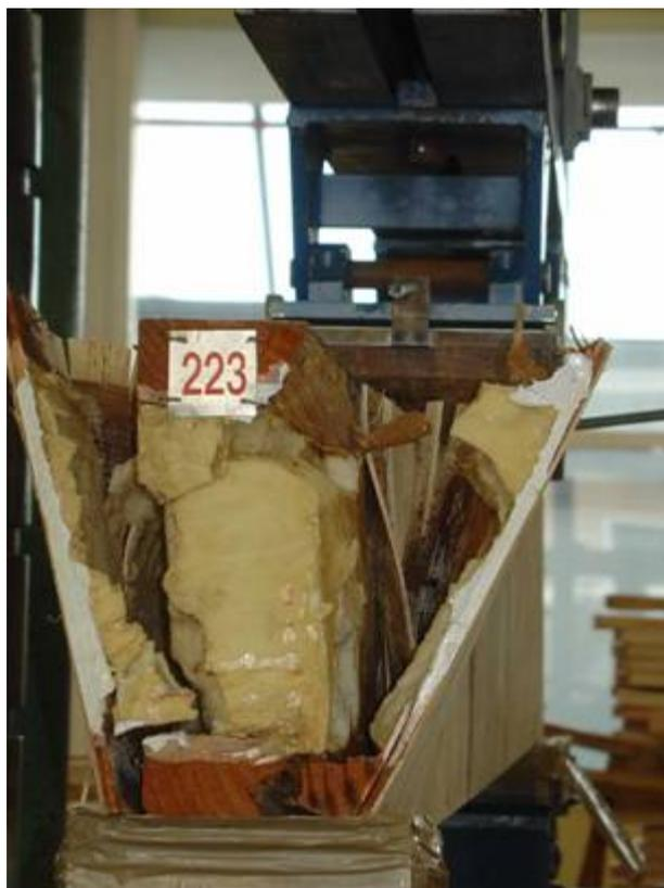
**Figure 9.10** Box beam with infill is failed under four point bending after exposure to 6 accelerated weathering cycles
