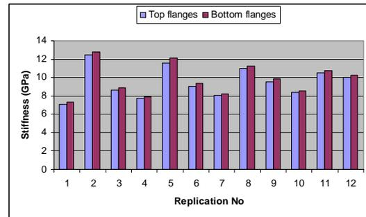
Filled Double I-beam-Distribution of MoE within top and bottom flanges
