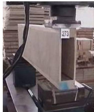
**Figure 6.4. Test arrangement for measuring maximum bearing capacity of the beams**
