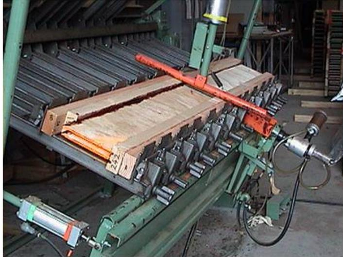
**Figure 3.10 Pneumatic press clamp (Taylor clamp)**
