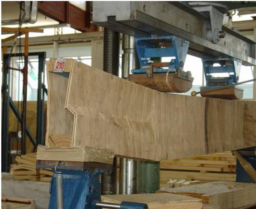
Figure 9.9 Box beam failed under four point bending test after exposure to 6 cycles of accelerated weathering conditions.
