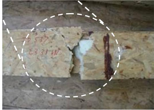
b) Flexural failure in Box I-beam
