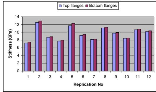
Filled Recessed beam-Distribution of MoE within top and bottom flanges
