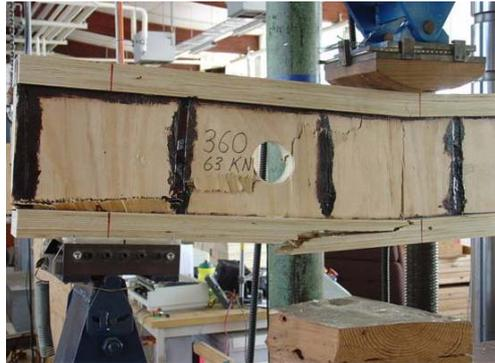
d) Filled LVL Double I-beam with web opening of 76mm
