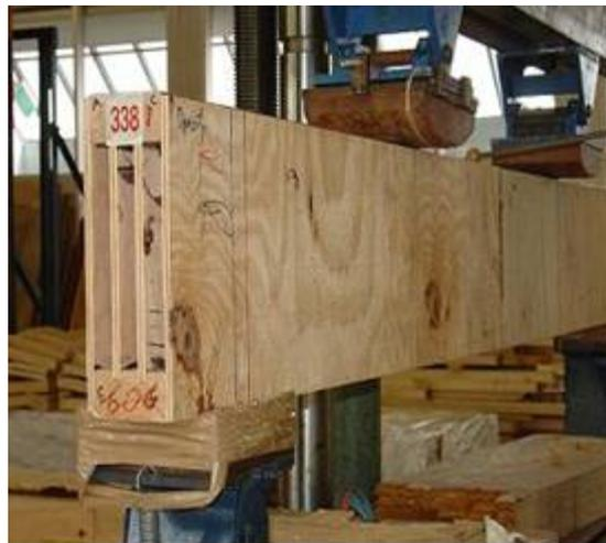
c) Boxed Double I-beam under four-point-bending
