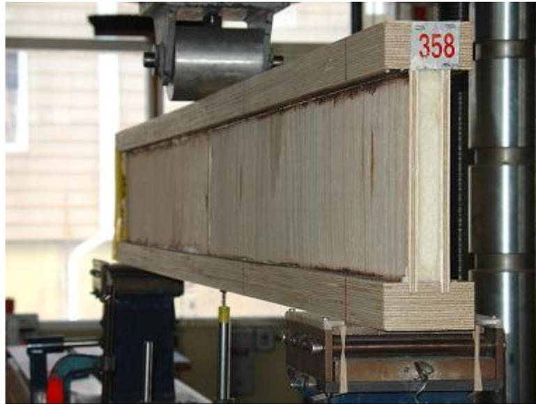
b) Testing filled LVL double I-beam under three point bending
