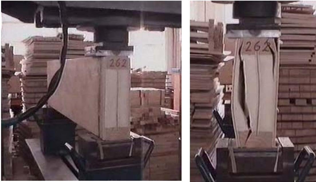
**Figure 9.2 Filled box I-beam before and after compression test**
