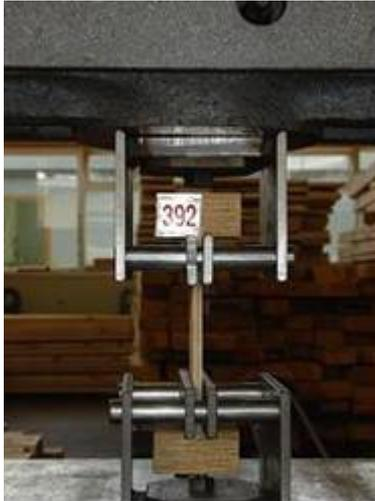
a) Testing apparatus used to measure pulling resistance of (LVL)I-beam
