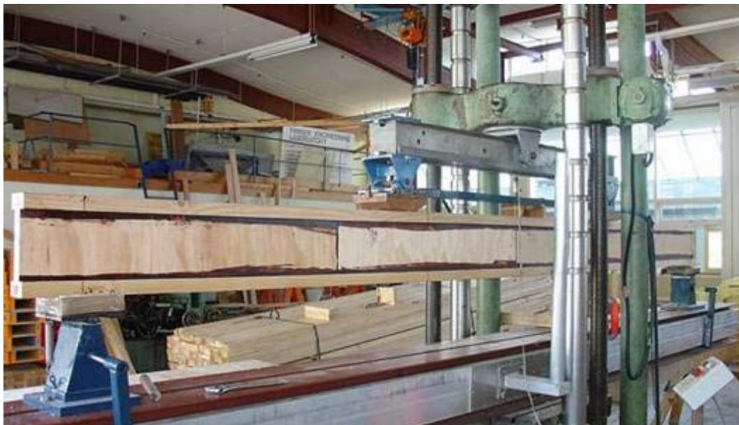
(b) Measuring MoE in bending for double I-beam
