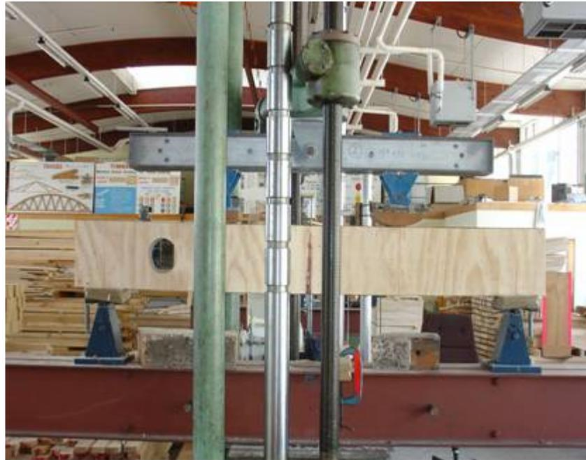
b) Filled Box I-beam with web opening of 152 mm
