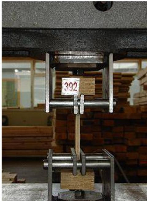
(a) Testing the pulling resistance of an I-Beam
