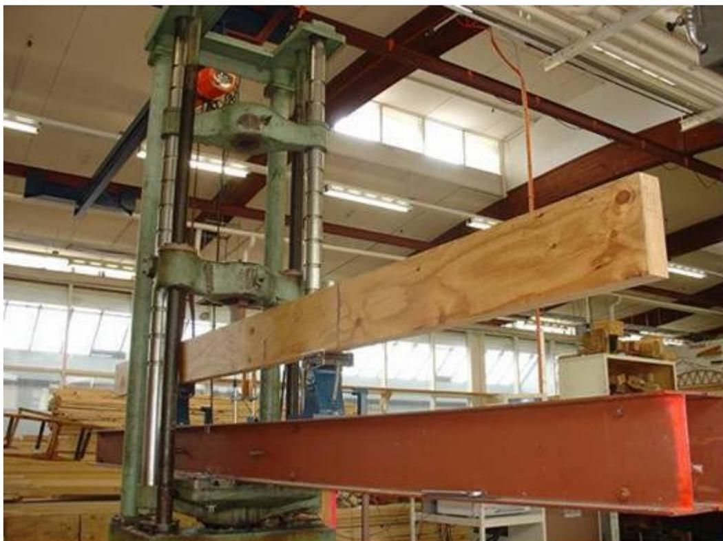
**Figure 4.10(B) LVL section subjected to three-point-bending over a 1450mm span**
