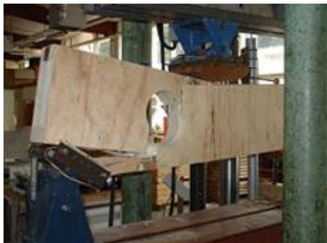
c) Filled Box I-beam after failure
