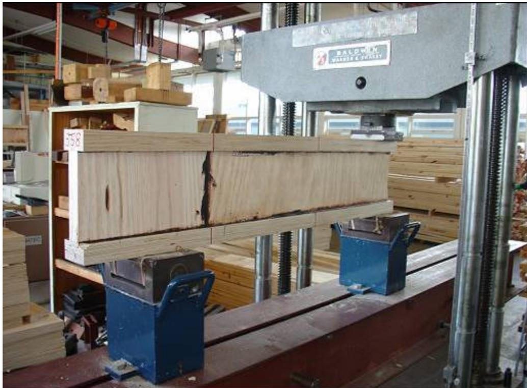
(b) Filled Double I-beam under bearing test
