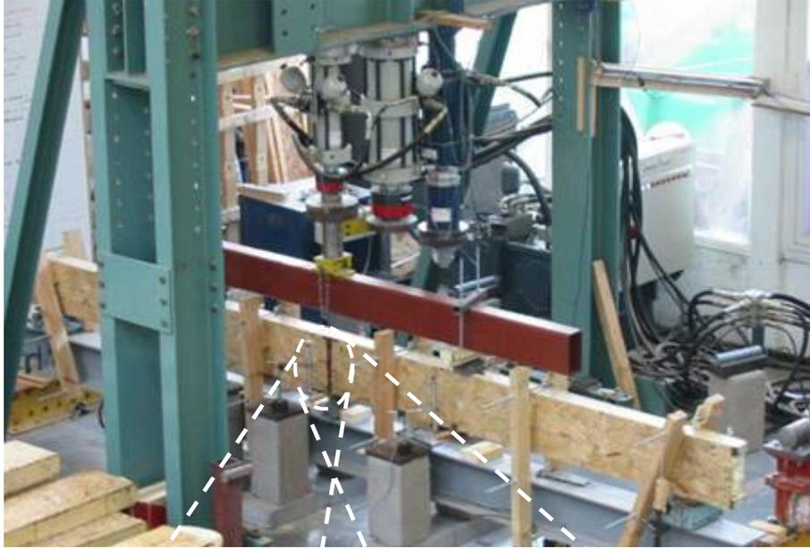
a) Destructive test, four point bending
