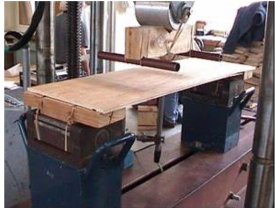
b) Testing modulus of elasticity
