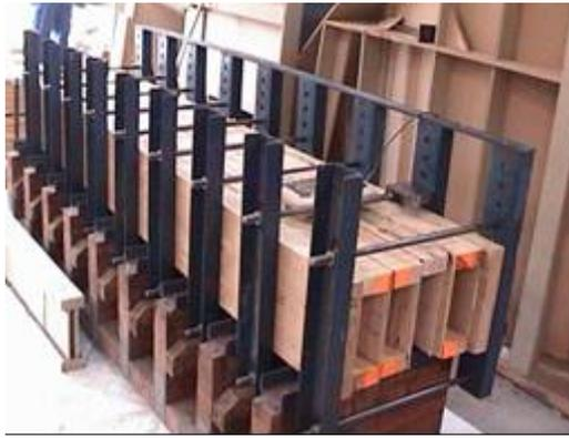
a) Box beam under the clamp
