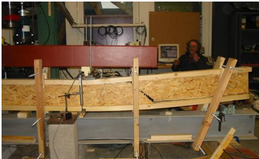
**Figure 9.15 Failure in an I-beam**
