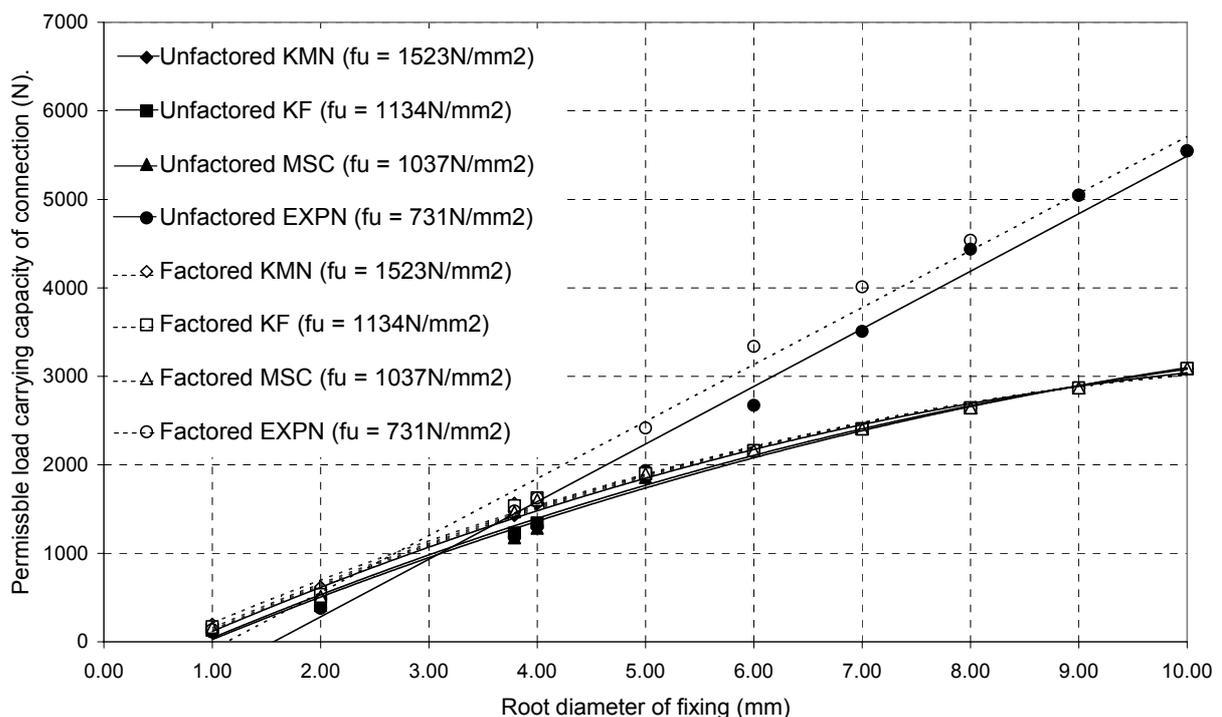
Figure 5 Un-factored calculated connection strength for a range of fixing diameters
