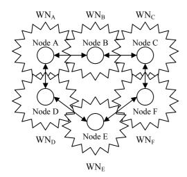
Figure 3: Passing network traffic to adjacent WNs
