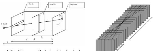
A Two-Slit camera. The horizontal and vertical slits define a unique ray for each scene point
