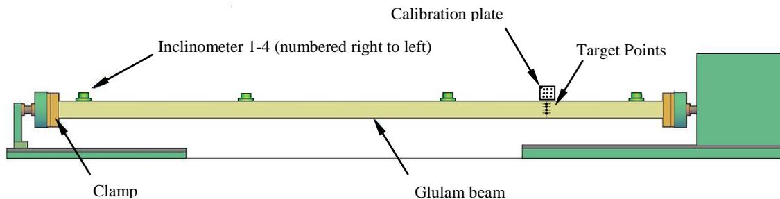
Figure 3 Schematic diagram for test setup timber joist
