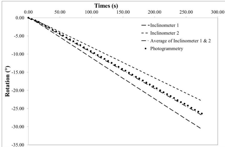
Figure 5 Comparison of the inclinometer and photogrammetric measurement for Sample 2
