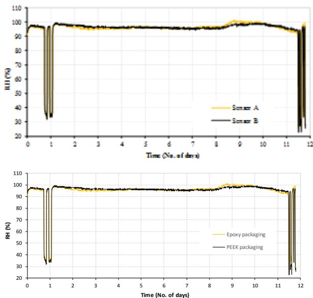
Figure 6: Performance of sensors with different polymeric packaging.
