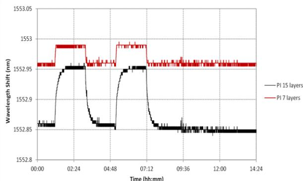
Figure 7 Effect of the thickness of the humidity sensitive polymer on sensor response
