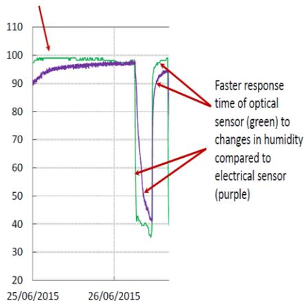
Figure 9: Detailed response time comparison between the photonic and electrical sensors
