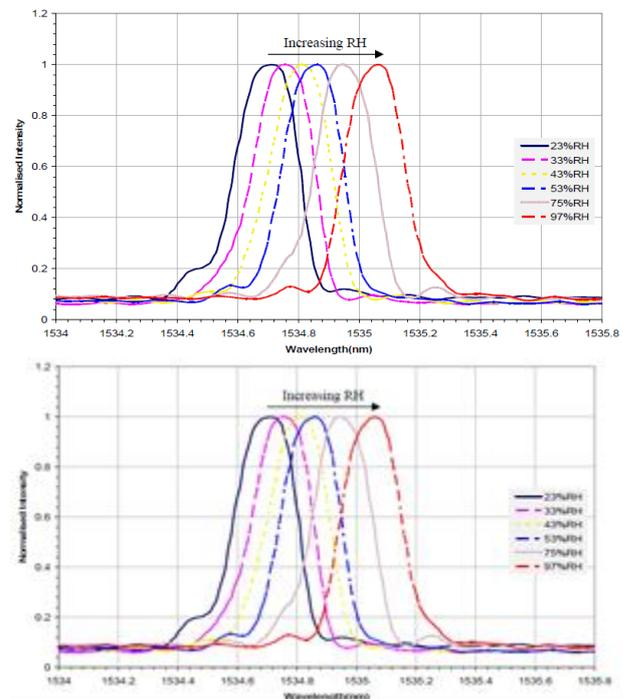
Figure 3: Reflection spectra of PI coated FBG sensor at different humidity levels
