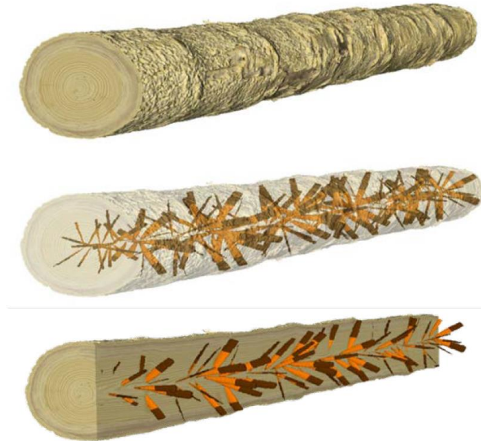
Figure 5 —Roundwood sawing optimisation according to X-ray based computed tomography; (Bruechert et al. 2017)
