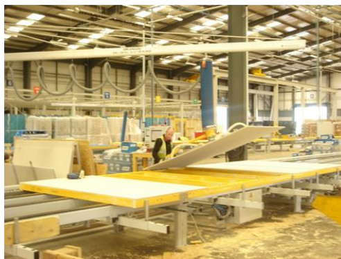
FIGURE 2.6 Plasterboard sheathing being added to the timber frames.
