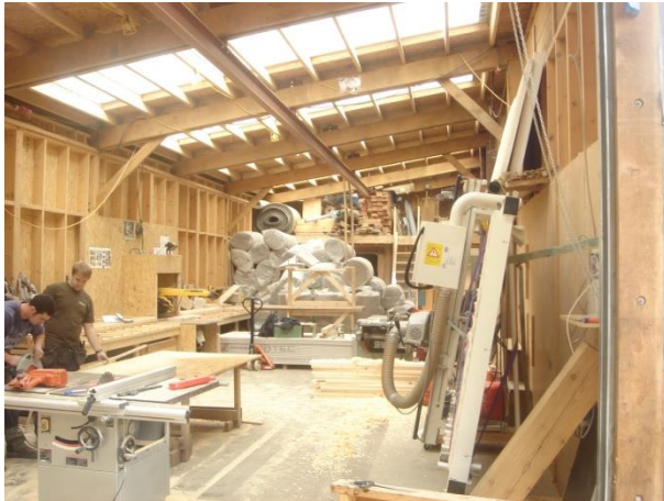
FIGURE 2.11 Example of smaller manufacturing facilities with a manual production process (MAKAR, Inverness).
