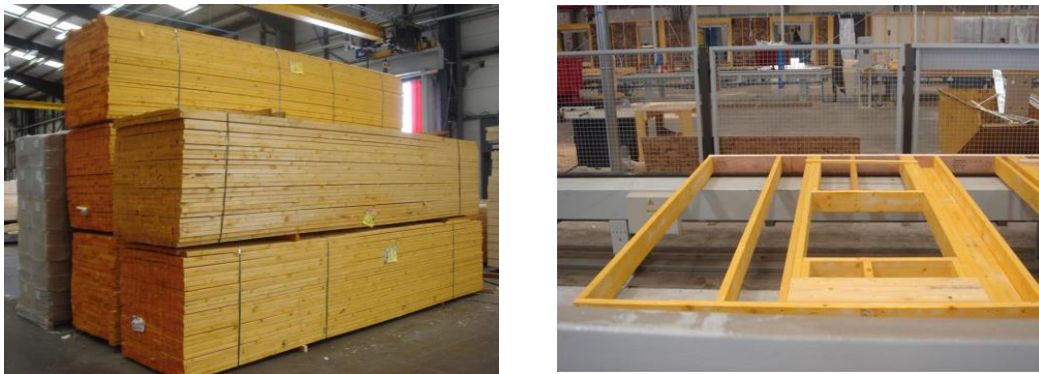
FIGURE 2.5 Offsite manufacturing of timber-frame panels at CCG (OSM) Ltd, Glasgow.
