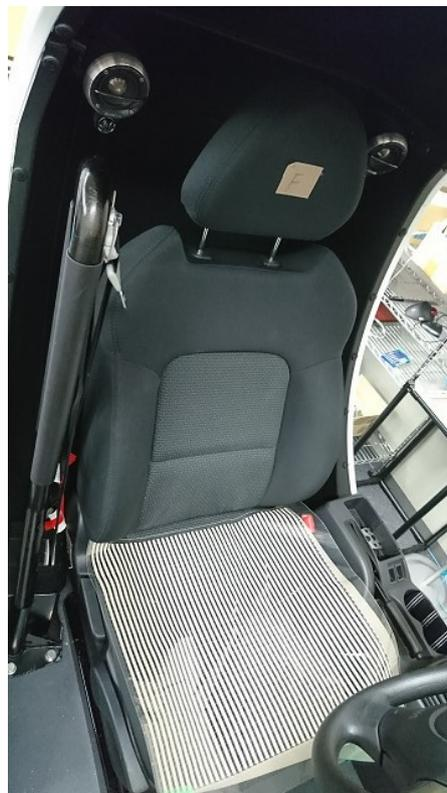
Figure 12 Body pressure mat on the seat of driving simulator
