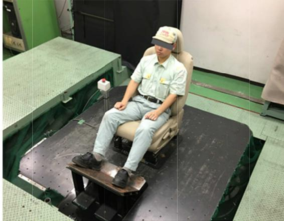
Fig.6 Laboratory apparatus for lateral human body shaking evaluation
