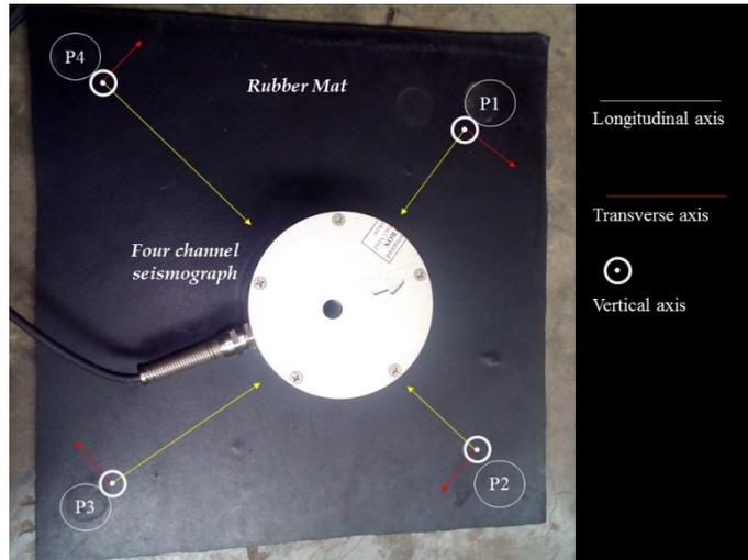
Figure 2: Experimental setup used to obtain the damping properties of rubber mat
