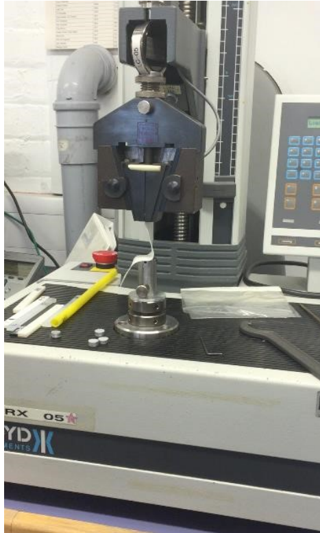
Figure 8. Peel test equipment and 'button' samples, 2016
