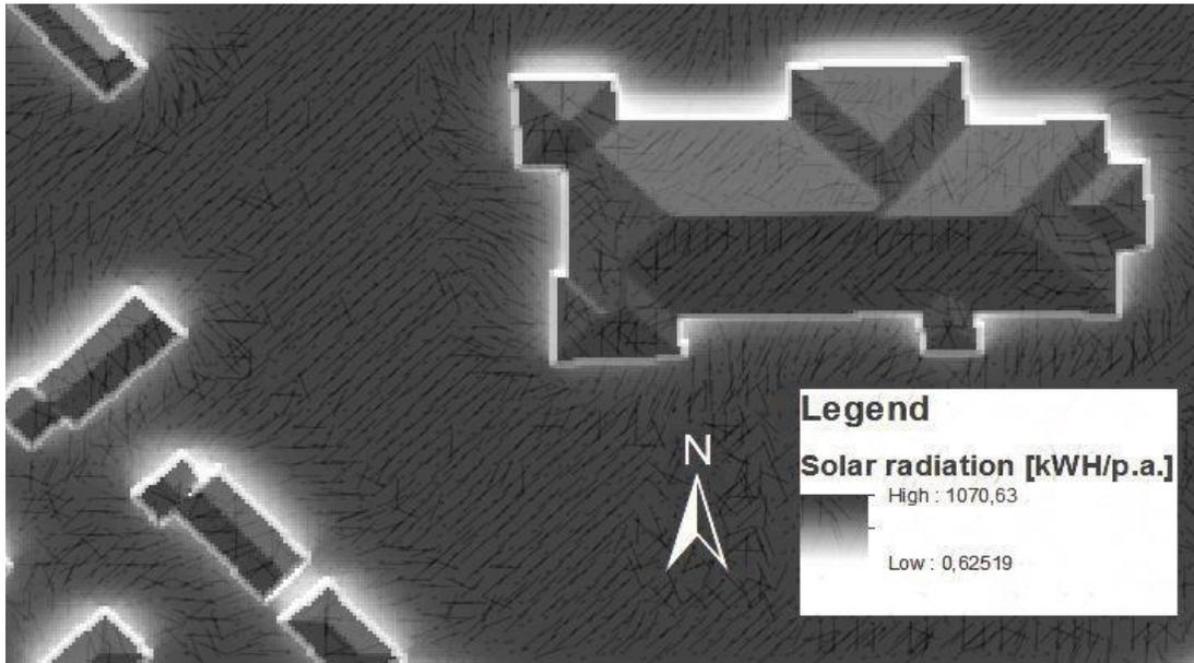
**Figure 43:** Extract of the solar energy raster displaying the calculated yearly solar radiation.
