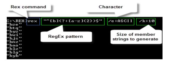
**Figure 6-8 Running Rex command utility against a constraint**: A figure demonstrating running Rex command against a defined RegEx constraint to generate the possible related member strings as shown in Table 6-3.
