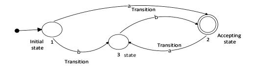
Figure 2-8 FSA illustrating transition state walks
