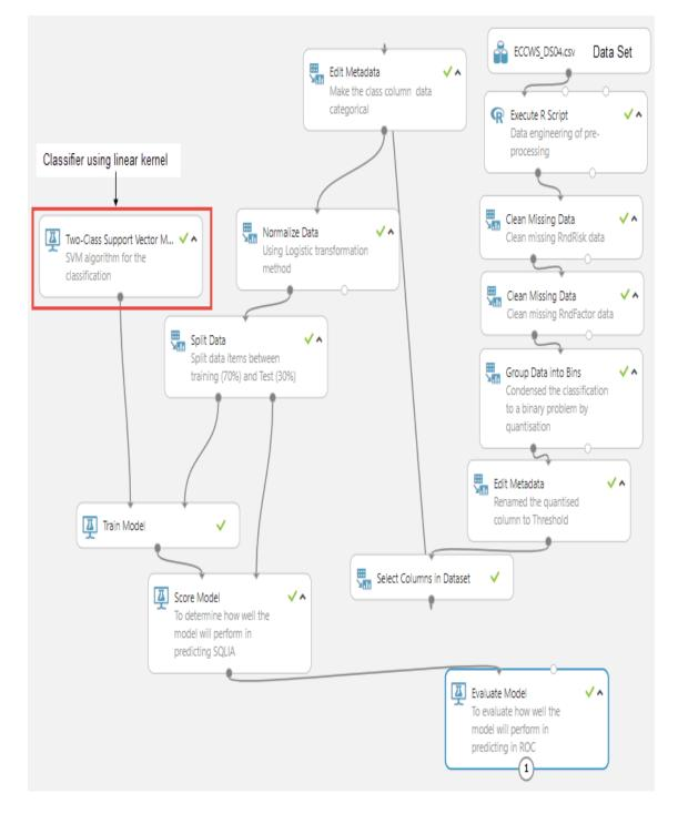
**Figure 4-8 The MAML studio predictive experiment**: The figure is a screen capture of MAML studio to illustrates experimental steps for the proposed model.
