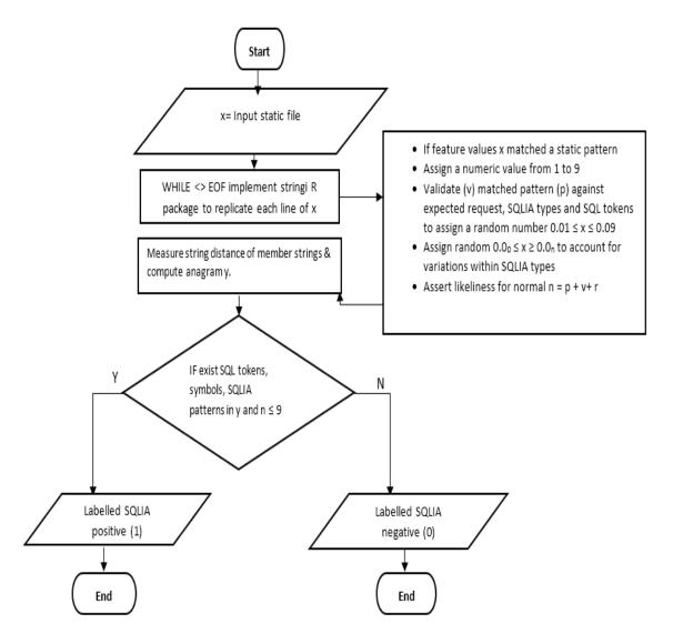
**Figure 4-6 A flowchart of the numerical encoding of features**: A Flowchart illustrating numeric encoding of features to obtain scalar numeric values required to train a supervised learning model.
