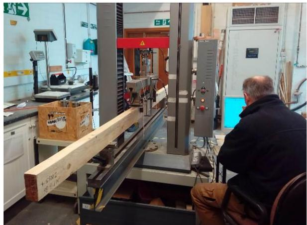
Figure 4. Bending test of a batten.
