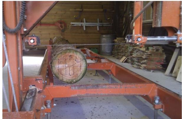
Figure 3. Sawmilling of a log.
