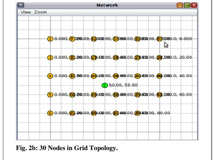
Fig. 2b: 30 Nodes in Grid Topology.
