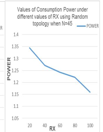
**Fig. 30: Power under different RX**
