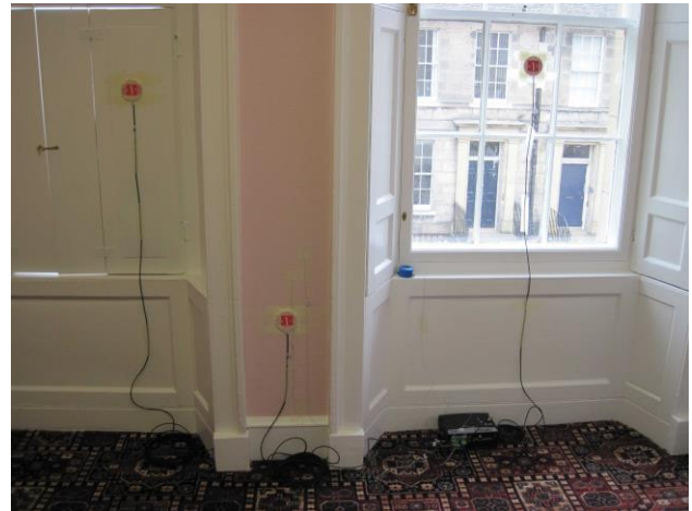
Fig. 9. In-situ test equipment on walls and windows
