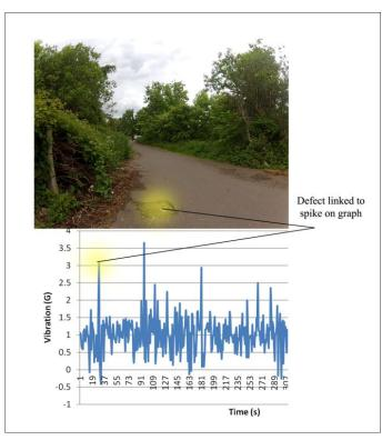
Fig.6 Vibration logger defect spike.
