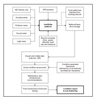
Fig.1 IntelliBike instrumentation and process flow diagram.
