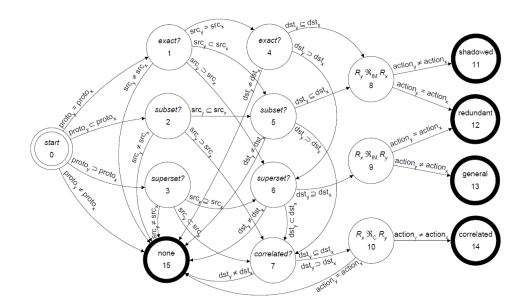
Figure 24: Anomaly state diagram from [9] for rules  $R_x$  and  $R_y$ , where  $R_x$  precedes  $R_y$  in the rules list.
