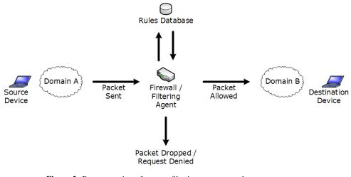
Figure 2: Representation of request filtering agent as analogous to a firewall.
