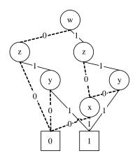
**Figure 8:** Reduced Binary Decision Diagram for the function  $f(w, x, y, z) = (w \land x) \lor (y \land z)$  with variable ordering of w, z, y, x.
