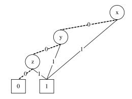
Figure 6: Reduced Binary Decision Diagram for the function  $f(x, y, z) = (x \lor y \lor z).$
