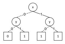
**Figure 3:** Binary decision diagram for the function  $f(x, y) = (x \lor y)$ .
