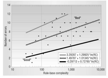
Figure 1: Number of errors as a function of rule-base complexity [3].
