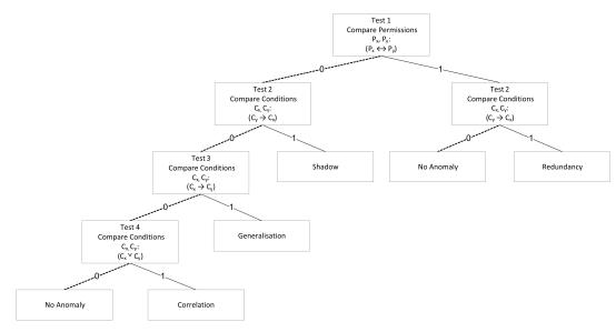
Figure 25: Simplified anomaly classification method for functional verification.
