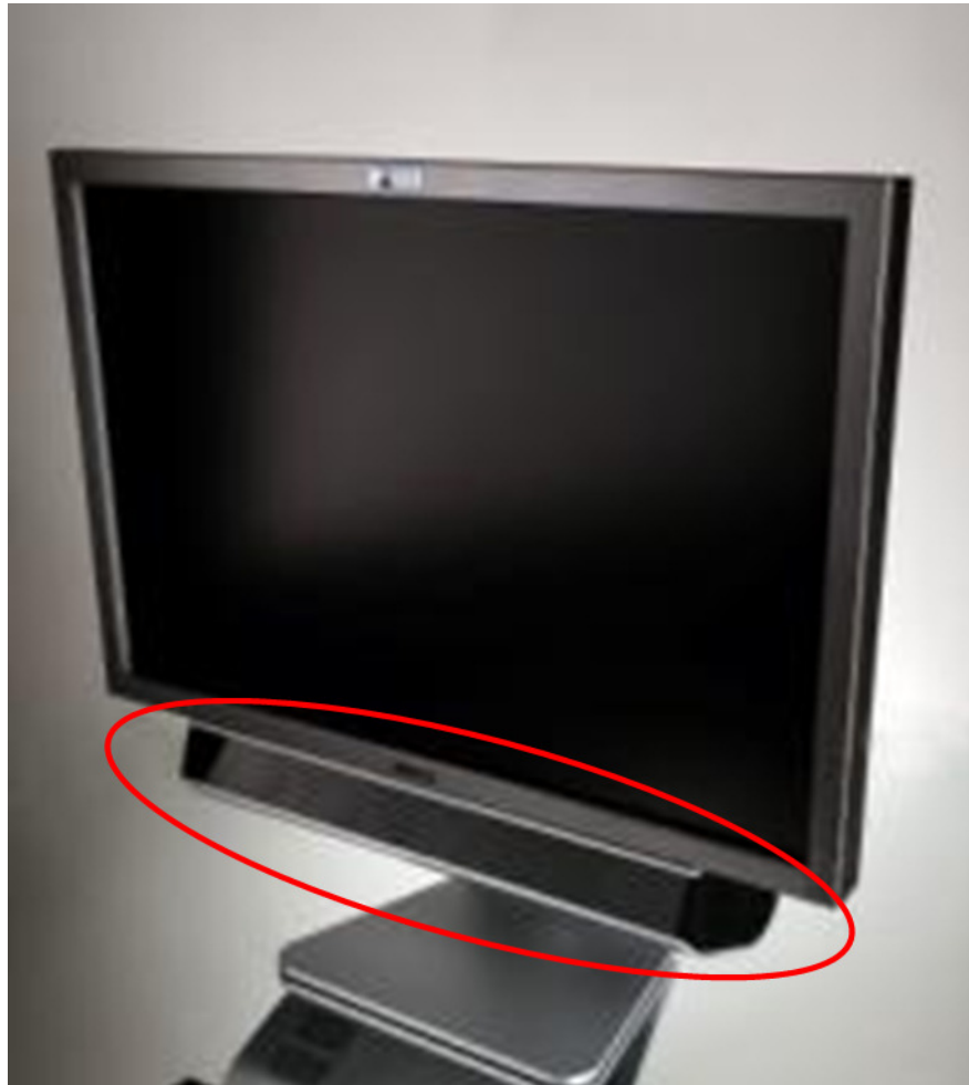
Figure 2.3. iView X RED eye tracker. The infra-red emitters and camera are housed in the device highlighted.
