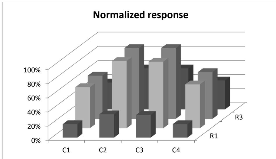
**Fig. 4.** Relative sensitivity of pixels in one array
