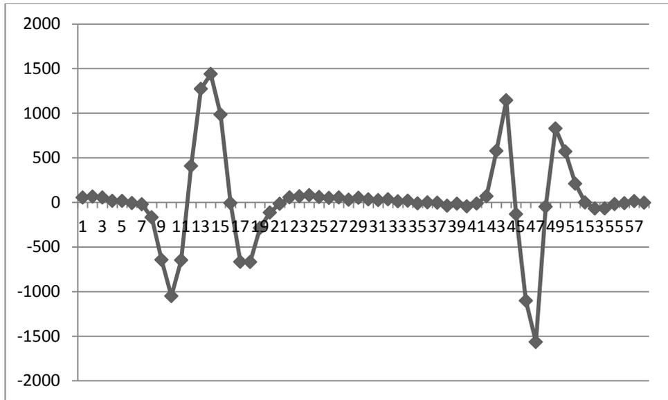
**Fig. 6.** Using the detector in differential mode to detect a hand swipe moving backwards and forwards across the detector.
