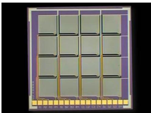
**Fig. 1.** 4x4 PIR Sensor Array (Source: [18]).
