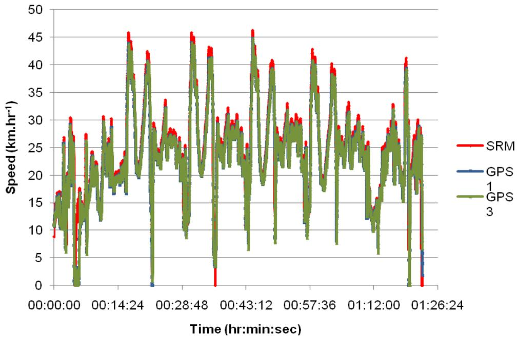
Figure x.1. Speed recorded during the full road trial from the GPS and SRM powermeter. The speed recorded by the SRM was significantly different to the speeds measured by the GPS units ( $p = 0.000$  for both). The speed recorded by the GPS units were not significantly different from each other ( $p = 0.485$ ).
