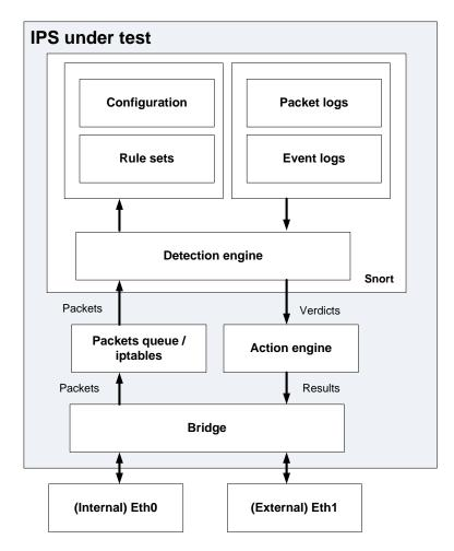
Figure 2: Schematic Implementation of the DUT
