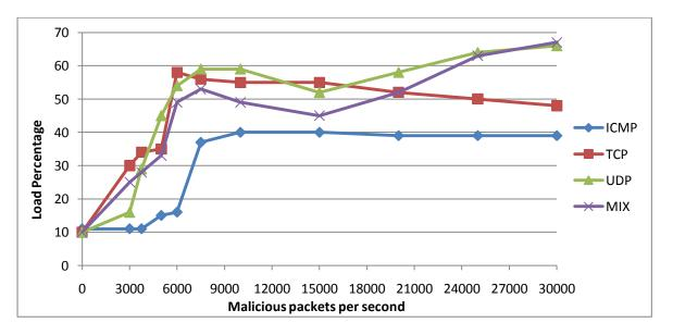
Figure 3: CPU Load Results
