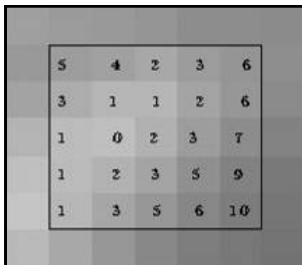
Figure 23: Grey shades are generated based on the scanned characteristics of a nonwoven sample. This allows the formation quality of the nonwoven to be analysed quantitatively.
