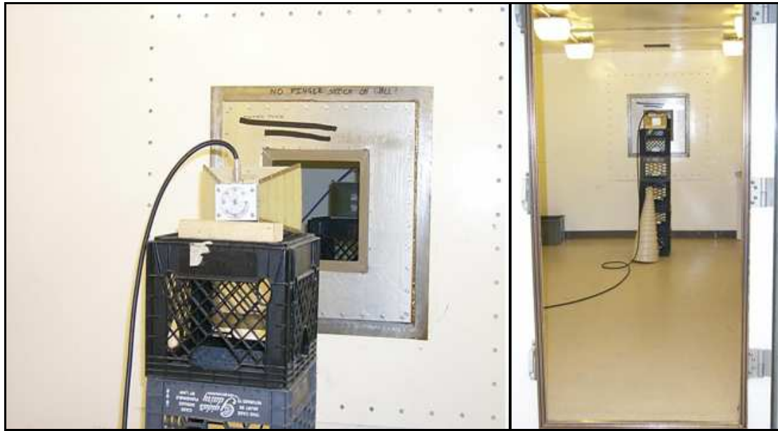
Figure 9: (Left) The MIL STD-285 method: The transmitting horn and material under test are seen. (Right) The image shows the shielded room in which the whole test setup is within. The walls are clad in a copper alloy lining and EMI gaskets have been applied to the door to prevent any external interference from affecting the results.
