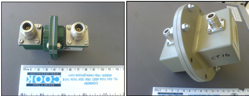
Figure 18: (Left) X-band waveguide transition, (Right) S-band waveguide transition.
