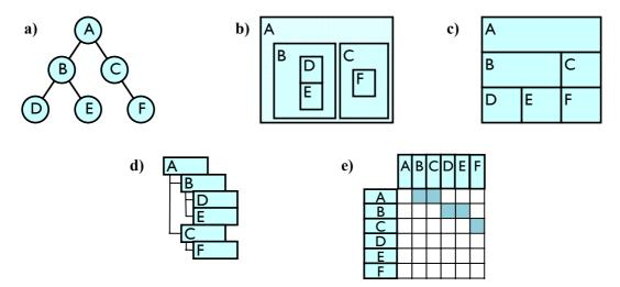
Figure 3. Basic types of tree representation - a) node-link, b) nested, c) adjacency, d) indented list & e) matrix representations
