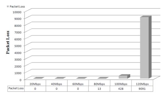
Figure 7 – Packet Loss Results
