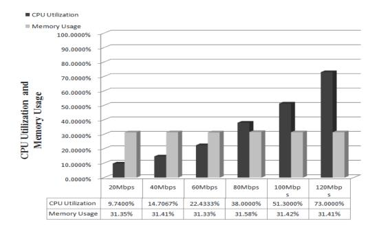
Figure 6 - CPU Utilisation and Memory Usage Results
