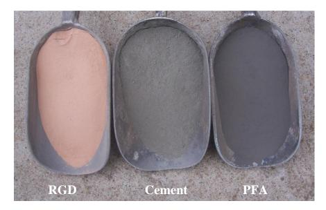
Fig. 7.15 RGD, cement and fly ash samples
