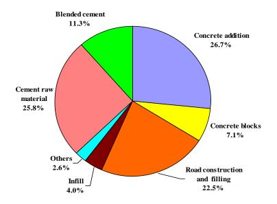
Fig. 2.8 Utilisation of PFA in the construction industry in Europe in 2004 (Ecoba 2006)
