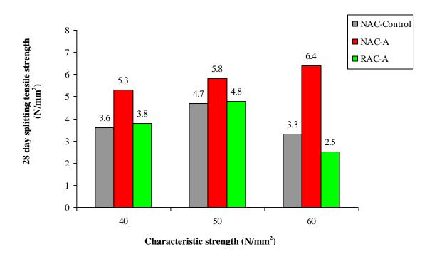
Fig. 5.7 Splitting tensile strength for NAC and RAC mixes of different grades
