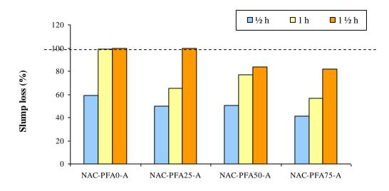
Fig. 4.22 Influence of PFA content on the rate of slump loss of NAC made with SP A
