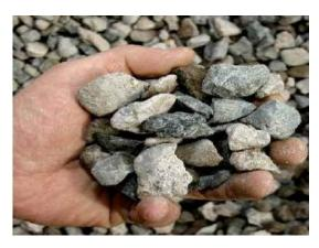
Fig. 2.5 The variability in shape, texture, and origin (seen simply by colour) of the RA
