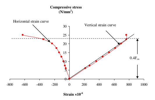
Fig. 7.11 Typical stress-strain curve for RAC specimen (RAC-CM)
