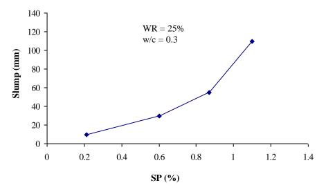
Fig. 4.27 Slump against SP relationship for a mix of 25% WR
