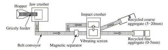
Fig. 2.17 Production plant for recycled aggregates (Kiyoshi 2007)
