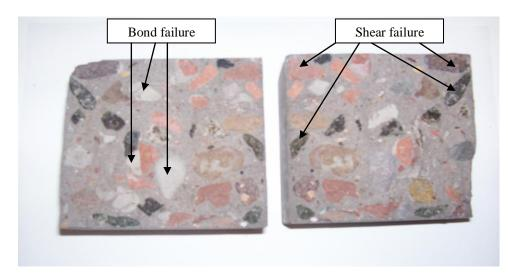
Fig. 5.11 Fracture surface of NA50-RA50 (blended aggregate concrete)
