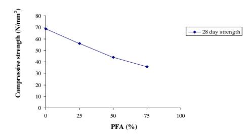
Fig. 6.1b Variation of the 28 day compressive strength of RAC with PFA content
