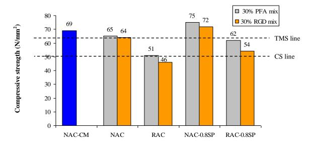
Fig. 7.29 Comparison of 28 day compressive strength of mixes with PFA and RGD
