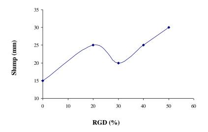
Fig. 7.16 Effect of RGD content on workability of NAC mixes
