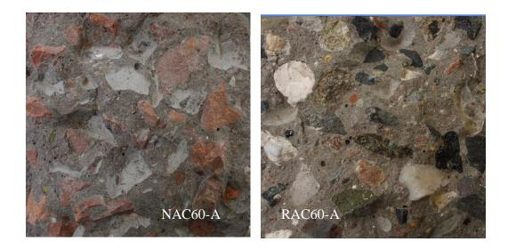
Fig. 5.10 Fracture surface of samples NAC 60-A and RAC 60-A
