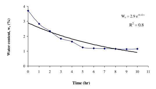
Fig. 4.8 Drying of NA over time
