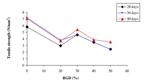
Fig. 7.20 Tensile strength of different RGD concretes at different ages
