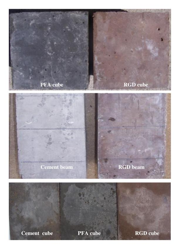
Fig. 7.23 Surface finish of RGD compared to cement and PFA concrete
