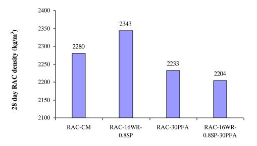
Fig. 7.13 Influence of PFA cement replacement on the bulk density of RAC concrete
