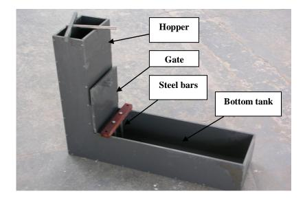
Fig. 8.4 L-box apparatus
