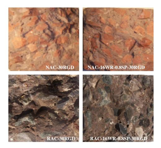
Fig. 7.24 Fracture surfaces of concrete samples with 30% RGD substitution
