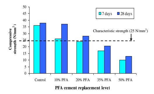
Fig. 3.3 Compressive strength of NAC concrete with various levels of PFA (Josette *et al.* 2006)
