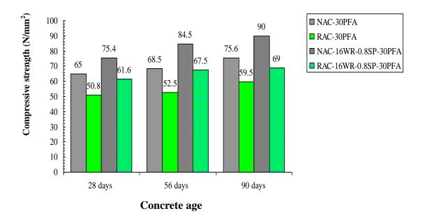
Fig. 7.4 Comparison of compressive strength of concrete with PFA at different ages
