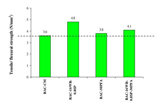
Fig. 7.5 Tensile strength of RAC with and without PFA compared to control mixes
