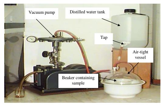
Fig. 4.7 Porosity testing apparatus
