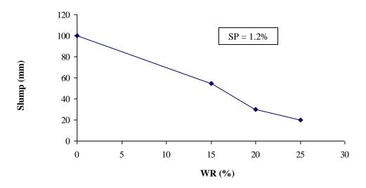
Fig. 4.31 Relationship between slump and WR for 1.2% SP
