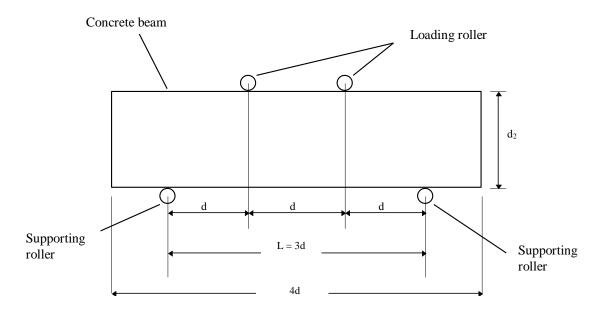
Fig. 5.3 Arrangement of loading test piece (two point loading)
