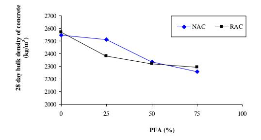
Fig. 6.10 Influence of PFA content on the density of concrete
