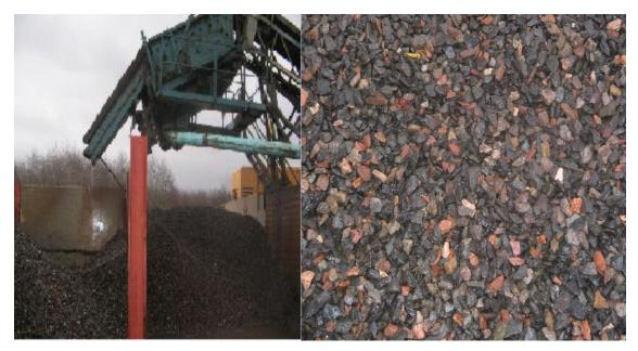
Fig. 2.14 Removing fines by washing with water
