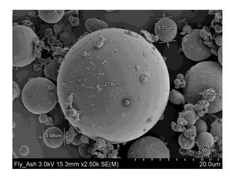
Fig. 4.12 SEM image of PFA specimen
