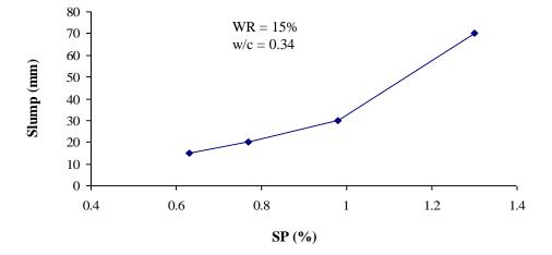
Fig. 4.25 Slump against SP relationship for a mix of 15% WR
