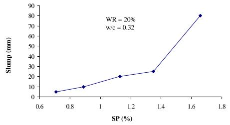
Fig. 4.26 Slump against SP relationship for a mix of 20% WR
