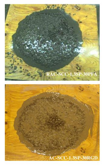
Fig. 8.8 Failed mixes due to segregation between coarse aggregate and cement paste although the mix passed the flow test
