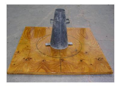
Fig. 8.2 Slump cone located on the inner circle above the base plate
