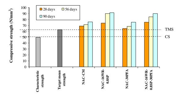
Fig. 7.2 Compressive strength of NAC mixes with PFA at different ages compared to control mixes
