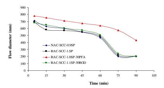
Fig. 8.14 Flow diameter against time
