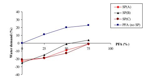
Fig. 4.20 Influence of SP type and PFA on water demand of binder paste
