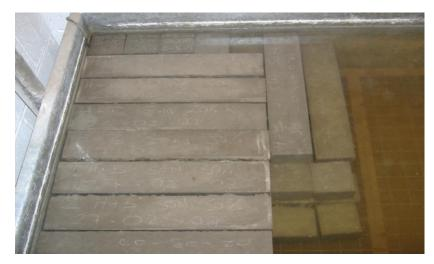
**Fig. 7.1** Beams and cubes kept in water tank at  $20 \pm 2^{\circ}$ C
