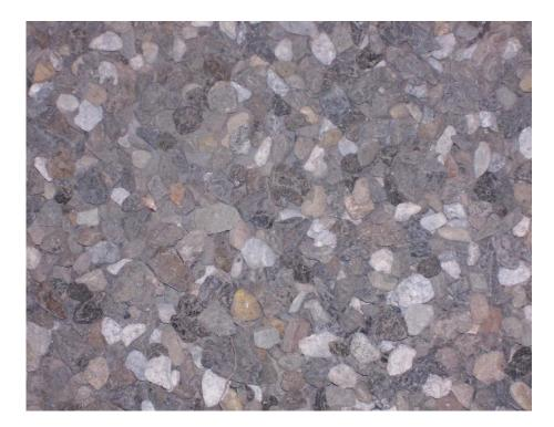
Fig. 2.15 Bowhill produced 20 mm coarse RA
