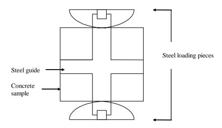
Fig. 5.1 Loading arrangement for tensile splitting strength
