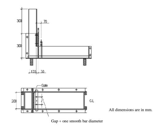
Fig. 8.3 Dimensions and typical design of L-box (EFNARC 2005)
