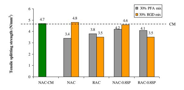
**Fig. 7.30** Comparison of tensile splitting strength of mixes with PFA and RGD and the 28 day control mix
