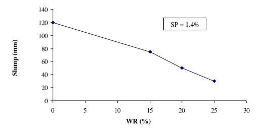
Fig. 4.32 Relationship between slump and WR for 1.4% SP
