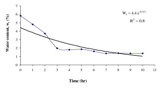
Fig. 4.9 Drying of RA over time
