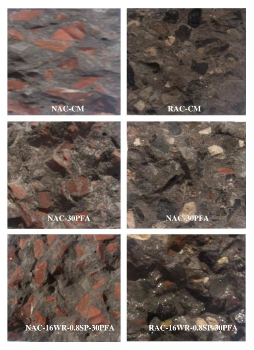
Fig. 7.7 Fracture surfaces of concrete samples
