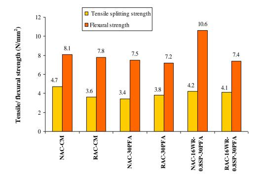
Fig. 7.6 Tensile splitting and flexural strength of mixes (NAC and RAC) with PFA compared to control mixes
