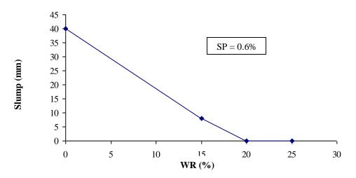
Fig. 4.28 Relationship between slump and WR for 0.6% SP
