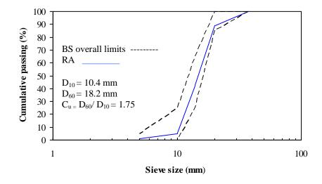
Fig. 4.3 Grading of recycled coarse aggregate
