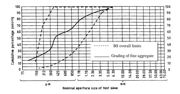
Fig. 4.4 Grading of fine concrete aggregate
