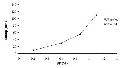
Fig. 4.24 Slump against SP relationship for control mix (0% WR)
