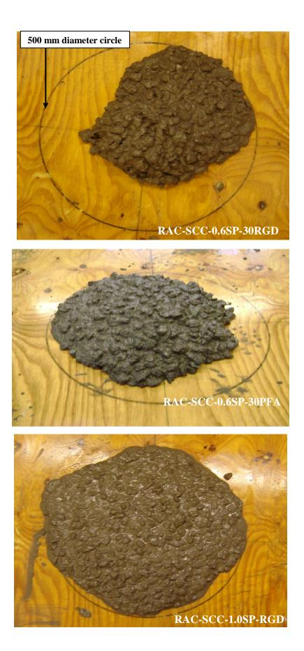
Fig. 8.7 Concrete failing the flow test
