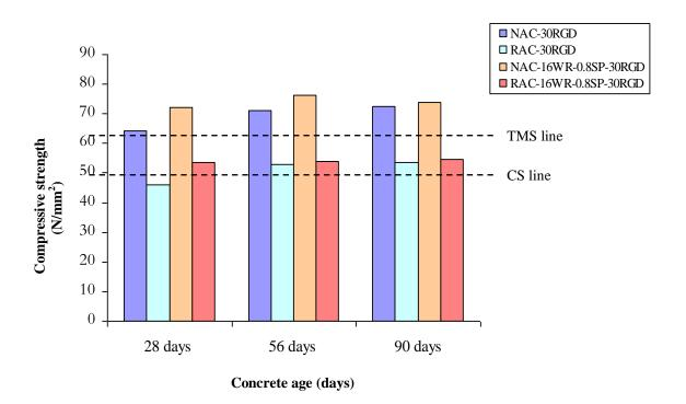
Fig. 7.25 Comparison of compressive strength of mixes with RGD at different ages
