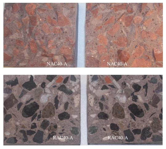
Fig. 5.8 Fracture surface of samples NAC 40-A and RAC 40-A
