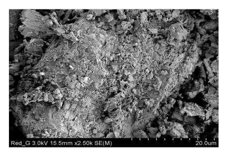
Fig. 4.14 SEM image of RGD specimen
