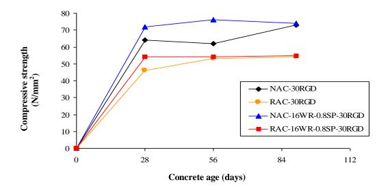
Fig. 7.26 Development of compressive strength of concrete mixes made with 30% RGD
