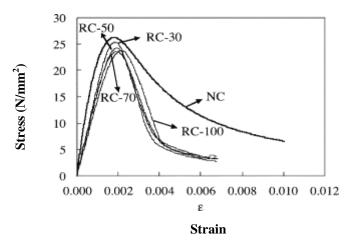
**Fig. 3.1** Typical stress-strain ( $\sigma$ - $\epsilon$ ) curves of RAC (Jianzhuang *et al.* 2005)
