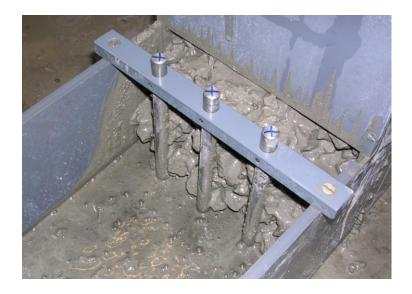
Fig 8.6 Blockages behind reinforcing bars
