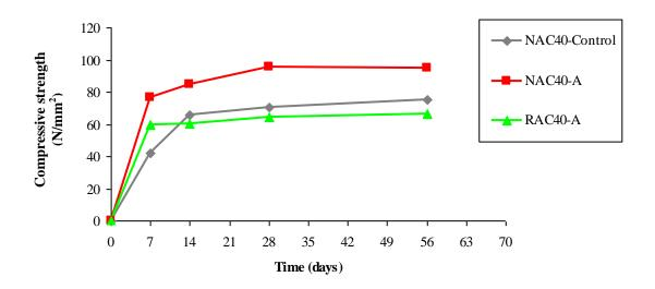
Fig. 5.5 Development of compressive strength of RAC as compared to NAC concrete
