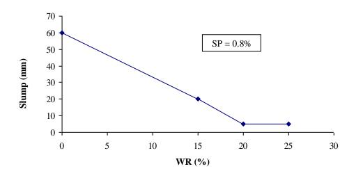
Fig. 4.29 Relationship between slump and WR for 0.8% SP
