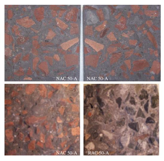
Fig. 5.9 Fracture surface of samples NAC 50-A and RAC 50-A
