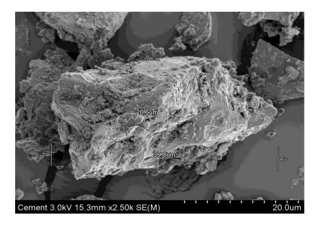
Fig. 4.10 SEM image of cement specimen
