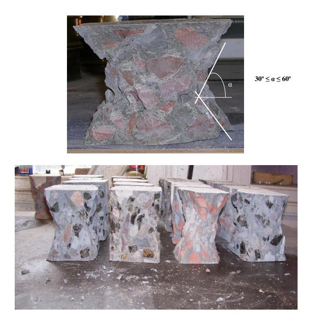
Fig. 6.8 The shape of crushed RAC and NAC concrete samples
