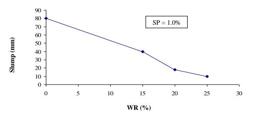
Fig. 4.30 Relationship between slump and WR for 1.0% SP
