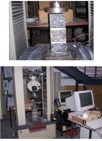
Type: Wire  $26ga - 19 \times 38 - 600V - 0.01PVC - 105C$  No 172619. Resistance of bridge circuit =  $120 \Omega$ . Gauge factor = 2.10. Dummy gauge not needed as it is a thermal compensating gauge. Load rate: 180 kN/minTest temperature:  $20 \pm 2^{\circ}C$  Cube size:  $100 \times 100 \times 100$  mm Jointing material: dental plaster
