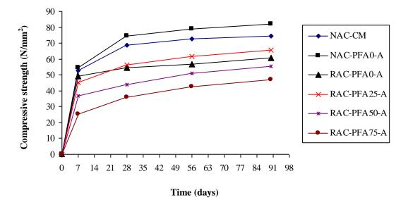
Fig. 6.1a Development of compressive strength of RAC with PFA replacing fine aggregate at different levels (SP type A used) compared to the control mix
