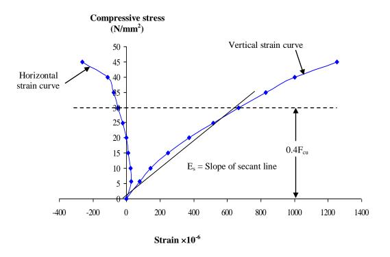
Fig. 7.10 Typical stress-strain curve for NAC specimen (NAC-CM)
