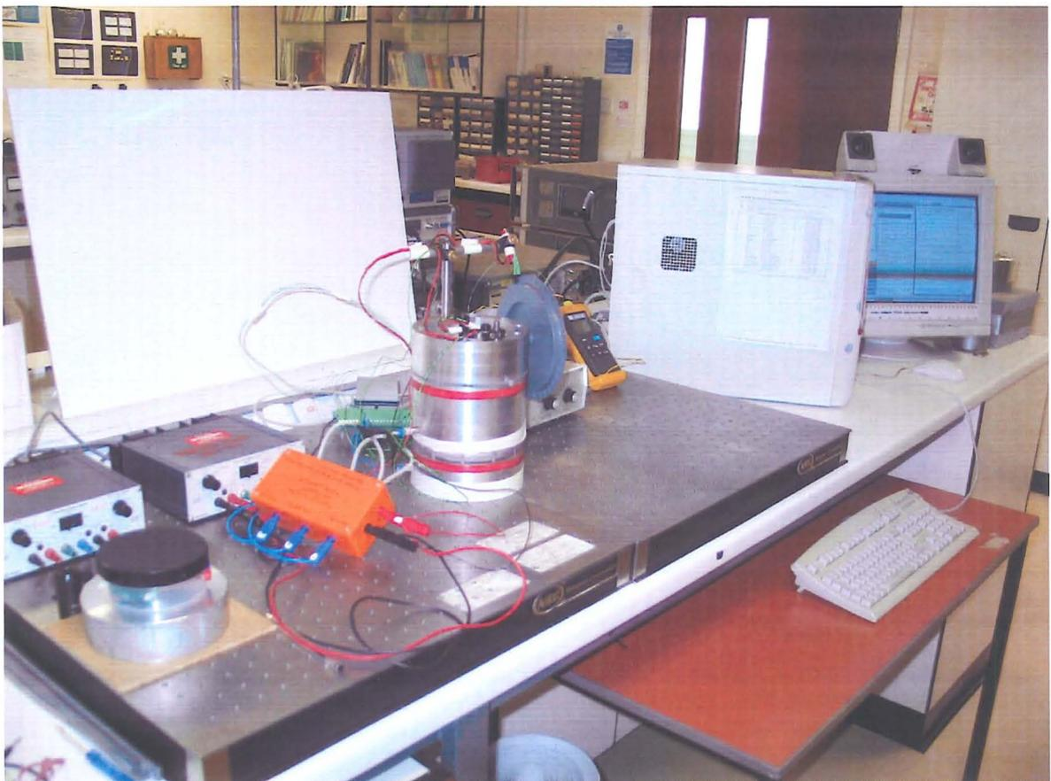
Figure 4.15 Test apparatus in laboratory, engine without insulating jacket.
