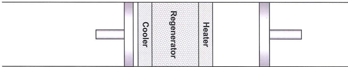
Figure 2.1 Stage 1 Isothermal expansion
