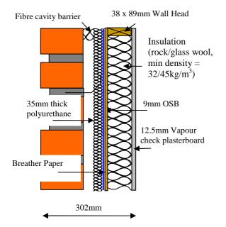
Detail 1: Cavity installed polyurethane insulation board
