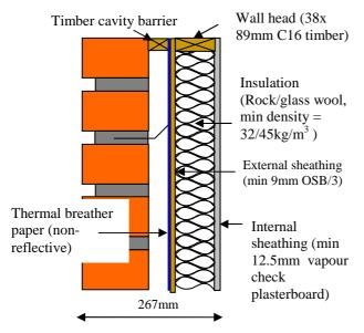
Figure 2: Standard timber frame wall detail
