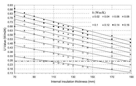
Figure 4: Relationship of wall detail U-value with internal insulation(between studs) thickness and  $\lambda$  value
