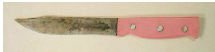
Figure 7. The knife handle is made from the plastic of an old bucket; the blade from a car panel
