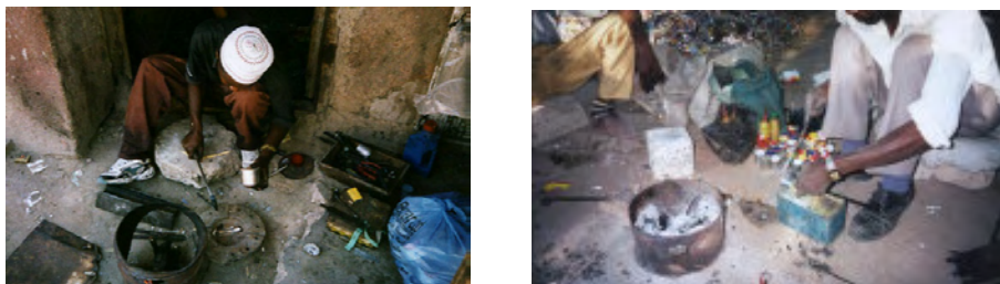
Figure 5. Local makers at the roadside use soldering irons to make kerosene lamps. One method uses a primus heater (left), the other a charcoal fire.
