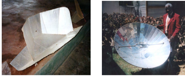
Figure 2. The Cookit (left) and Concave Reflector Cooker (right) with Pastor Fuataeli S.Muusi, Lutheran Church of Tanzania
