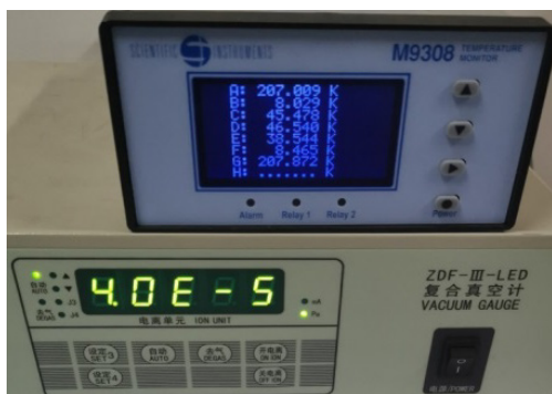
FIGURE 17. Measured the Cryogenic QRHF temperature results
