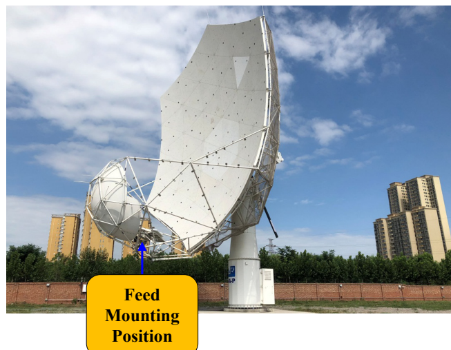
FIGURE 21. SKA dish prototype with location of the proposed feed.
