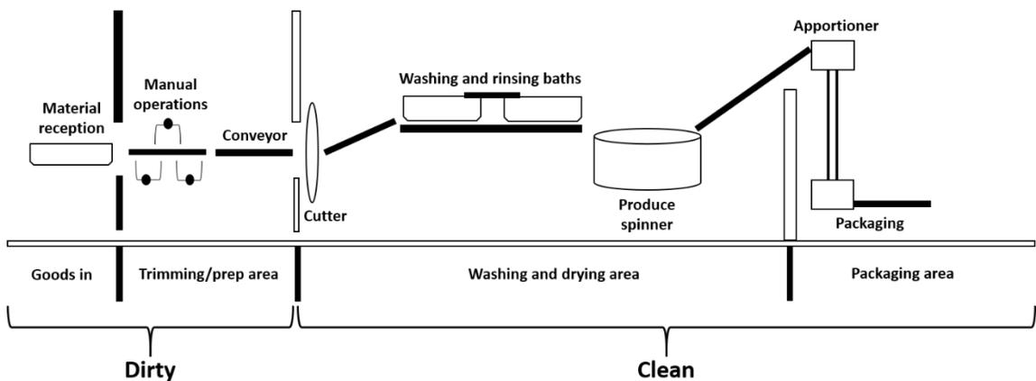
Figure 5.2. **Schematic of a fresh cut produce washing system.** Adapted from Allende and Artes (2005).
