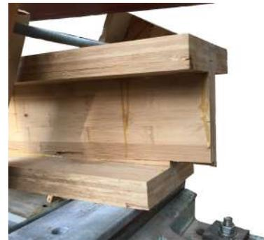
(b) Horizontal shear failure
