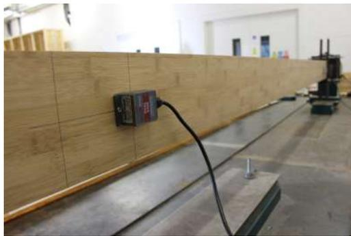
(a) The inclinometer attached on the beam
