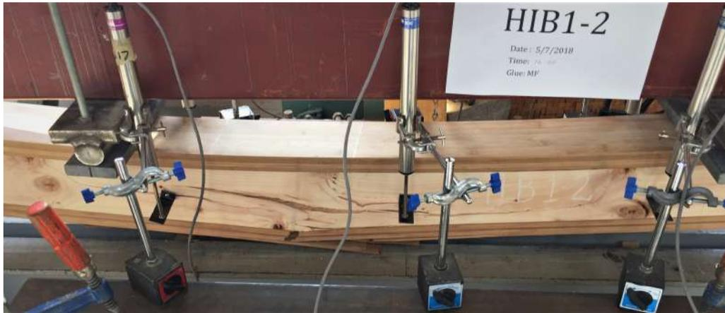
Figure 4.12: IBHB failed under flexural load
