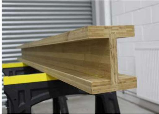
(a) Engineered Bamboo I-Beam (BIB)
