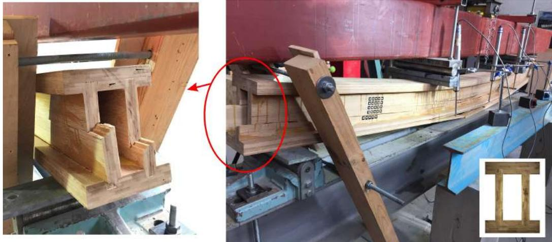
Figure 5.7: BDIB1 failure observations
