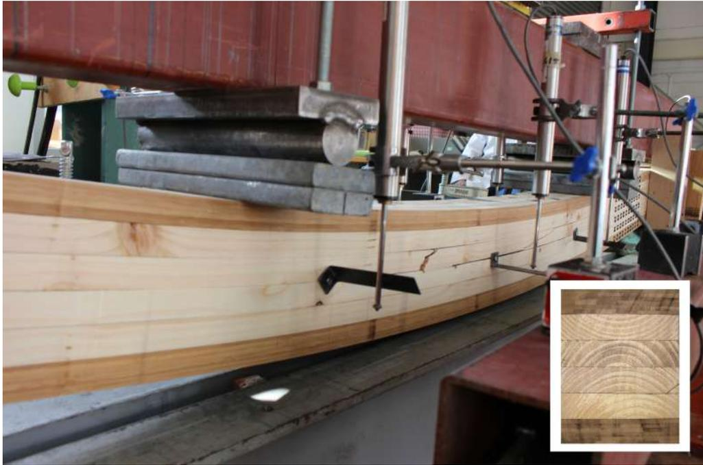
**Figure 4.11:** Bamboo sandwich beam failure
