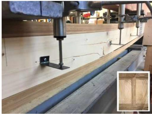
(a) Failed beam under the load
