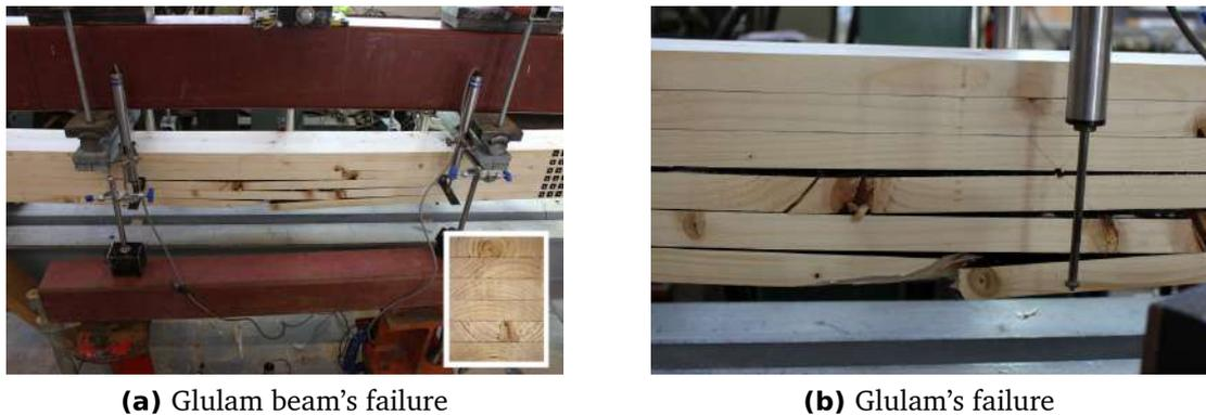
**Figure 4.10:** Glulam Beams' failure
