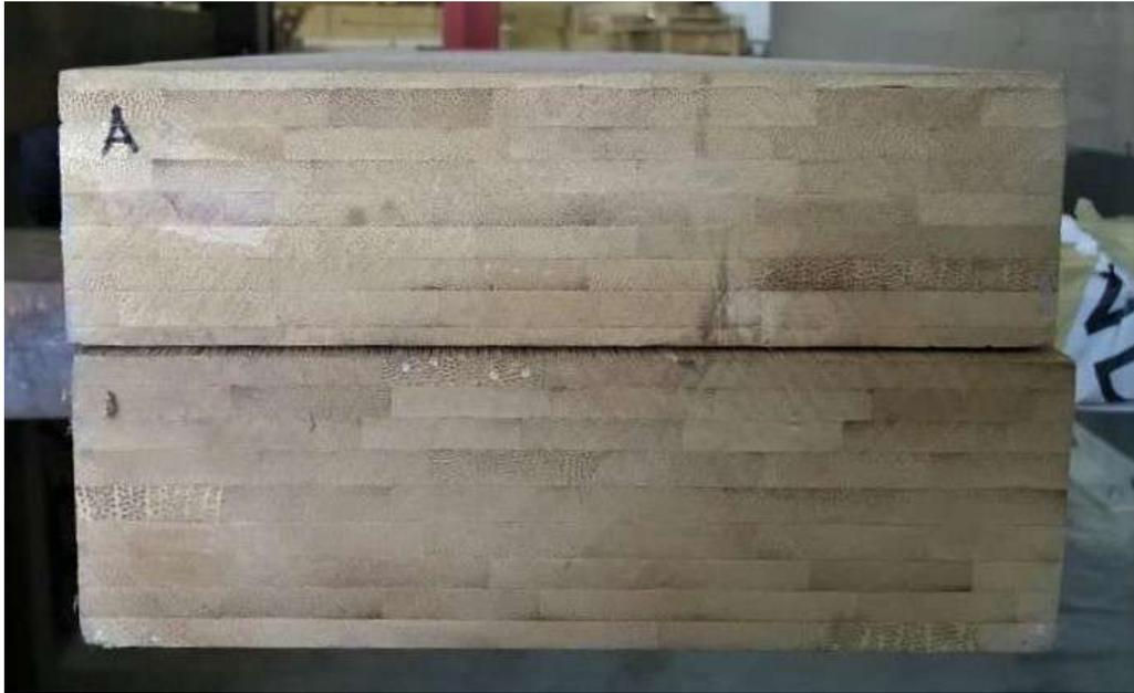
**Figure 2.6:** Laminated bamboo lumber cross-section
