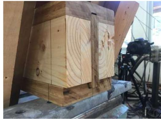
(b) Delamination of the beam at the flange connection
