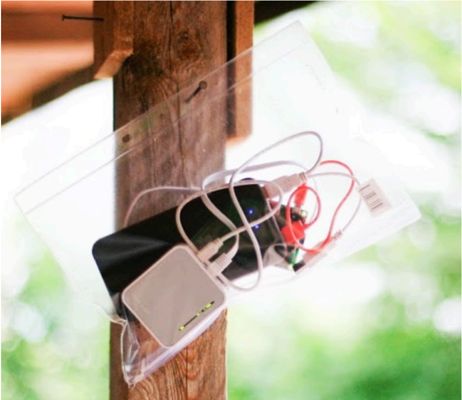
Figure 1: an early version of the WiFi network zone in an outdoor location, including the Raspberry Pi computer and battery.
