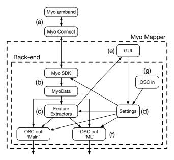
Figure 2: Myo Mapper's architecture.
