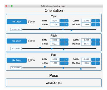
Figure 4: Myo Mapper's Calibration and scaling window.
