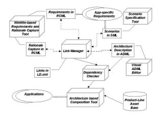
Figure 5. Prototype Tool Suite for Product Line Development
