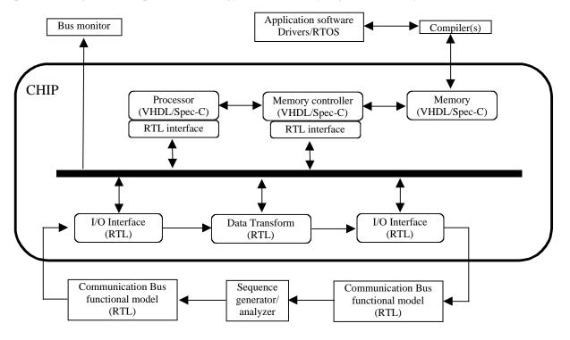
must completely describe the behavior of the system as a whole. The various components are typically specified using different specific technology as illustrated by Figure 5 [Keating and Bricaud 1999].
