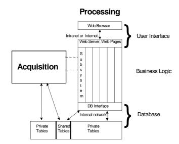
Figure 4. Three-tiered architecture.
