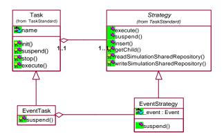
Figure 8: The TaskEvent framework in UML.
