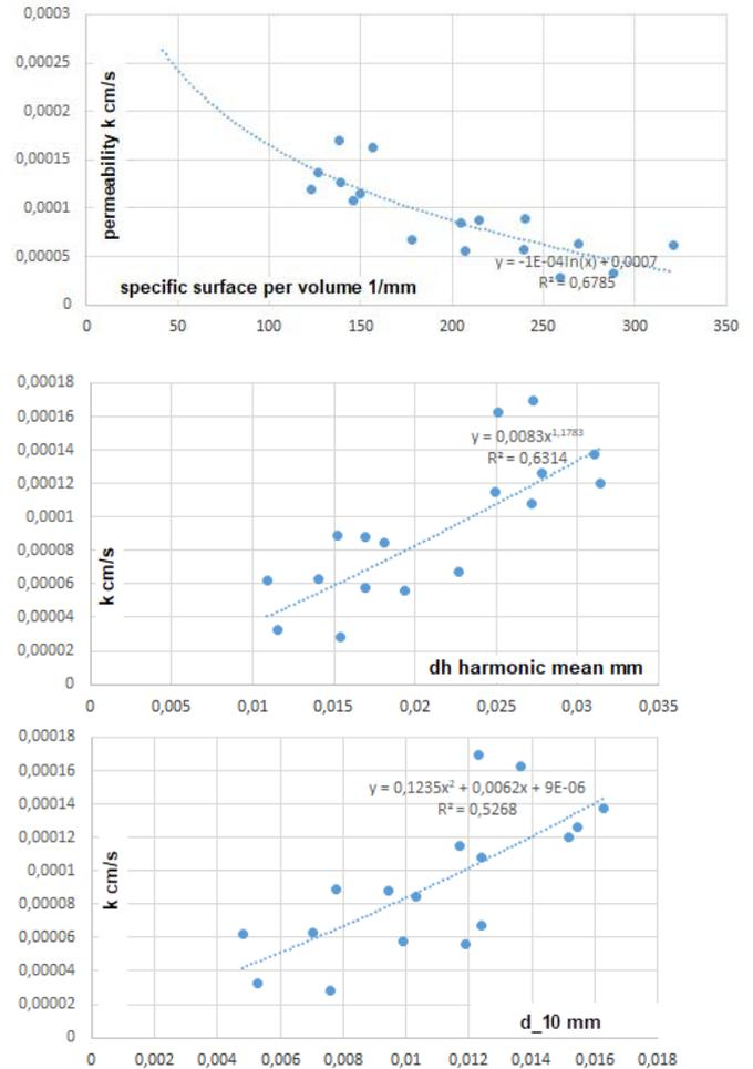
**Figure 19.** Re-evaluation of data series 2 of Nagy in terms of various diameter values specific surface parameter (containing density info), harmonic mean  $d_h$  and  $d_{10}$  with  $R^2=0.68, 0.63$  and  $0.52$  resp.).
