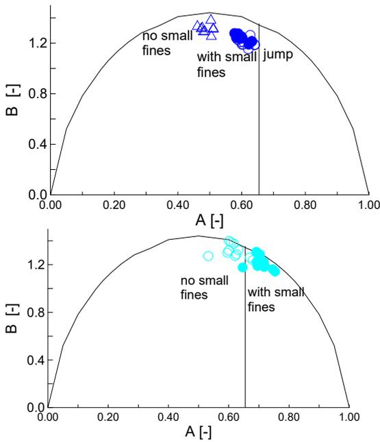
**Figure 6.** Effect of fines (gradation type 1 (dark blue) and 2 (light blue)) on the normalized and on the non-normalized entropy parameters. The open circles are by assuming smaller zero fractions up to the foregoing actual smallest limit (gave practically the same results as the Weibull data).
