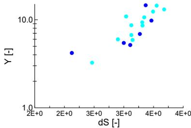
**Figure 12.** Relations with  $Y$  and the entropy increment parameter for PSDs of gradation types 1 (dark blue) and 2 (light blue) examined
