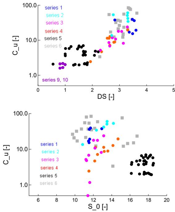
**Figure 10.** Relations with  $C_u=U$  for PSDs of gradation types 1 (dark blue) and 2 (light blue) examined with non-normalised entropy coordinates. The entropy increment  $\Delta S$  showed a univocal relation. The  $S_0$  regression was different for the various series.
