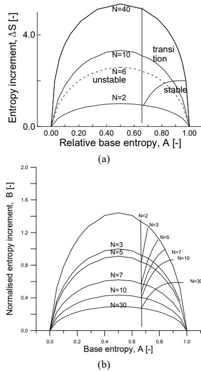
**Figure 2.** Internal or grain structure stability criterion (a) Partly normalized grading entropy diagram, the lines are the maximum lines (images of the optimal lines) for various  $N$  values. (b) The normalized grading entropy diagram for various  $N$ . The line related to transition zone is dependent on  $N$ .
