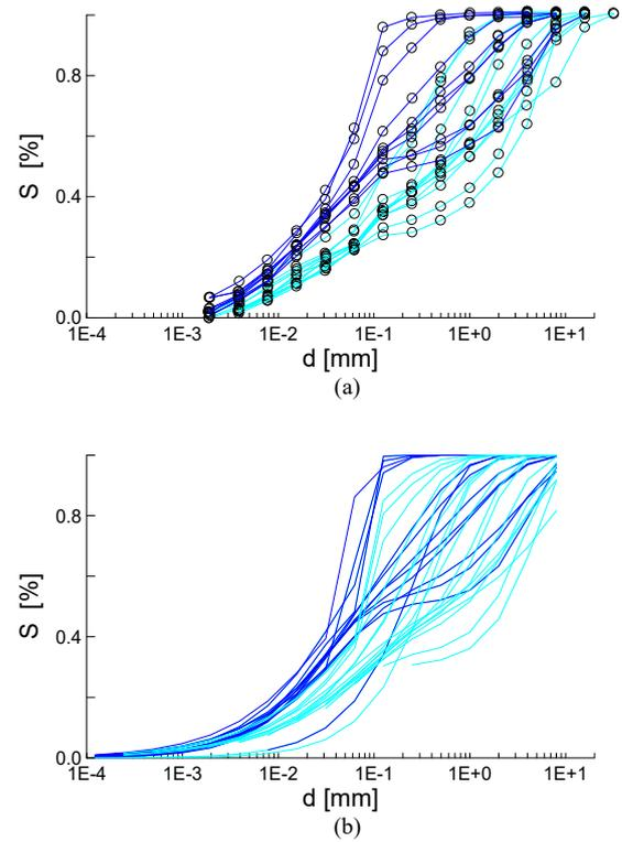
**Figure 4.** (a) Measured PSDs of gradation types 1 (dark blue) and 2 (light blue) examined. (b) Weibull fitted PSDs of gradation types 1 (dark blue) and 2 (light blue).
