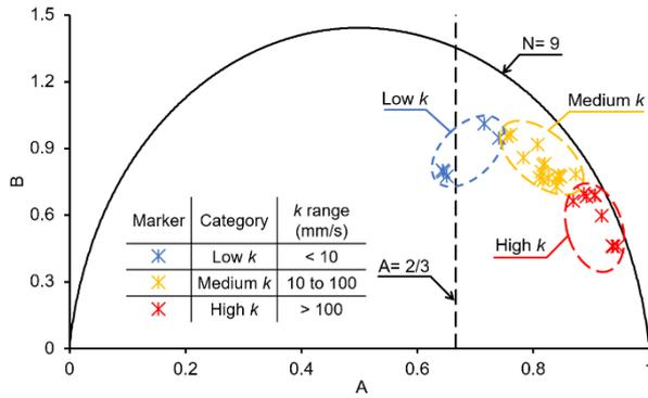
Figure 3. Identified permeability zones shown on the normalized entropy diagram (adapted from Feng et al, 2019a) [1]
