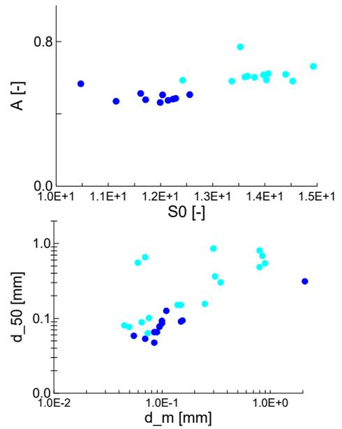
**Figure 13.** Relations of the two base entropy parameters and for the two empirical mean estimates  $d_{50}$  and  $d_m$ , for PSDs of gradation types 1 (dark blue) and 2 (light blue) examined
