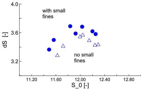
**Figure 7.** Effect of fines (gradation type 1 (dark blue) and 2 (light blue)) on the non-normalized entropy parameters (Series 1.2 -1.7, 1.10-1.11).
