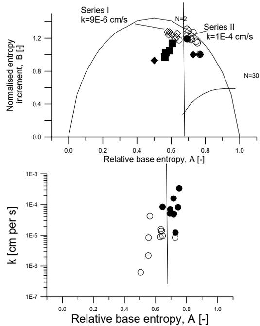
**Figure 14.** The mean falling head test data on pre-determined soil mixtures in the 2 series of measurements.
