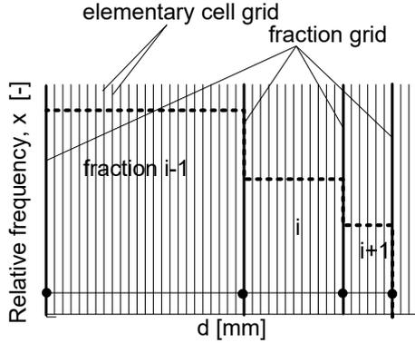
**Figure 1.** (a) Some grading curve parameters used in practice. (b) The grading density curve embedded in the elementary cell grid, assuming uniform distribution within the fractions.
