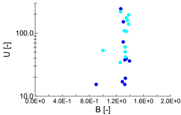
**Figure 11.** Relations with  $C_u=U$  for PSDs of gradation types 1 (dark blue) and 2 (light blue) examined with normalized entropy coordinates.
