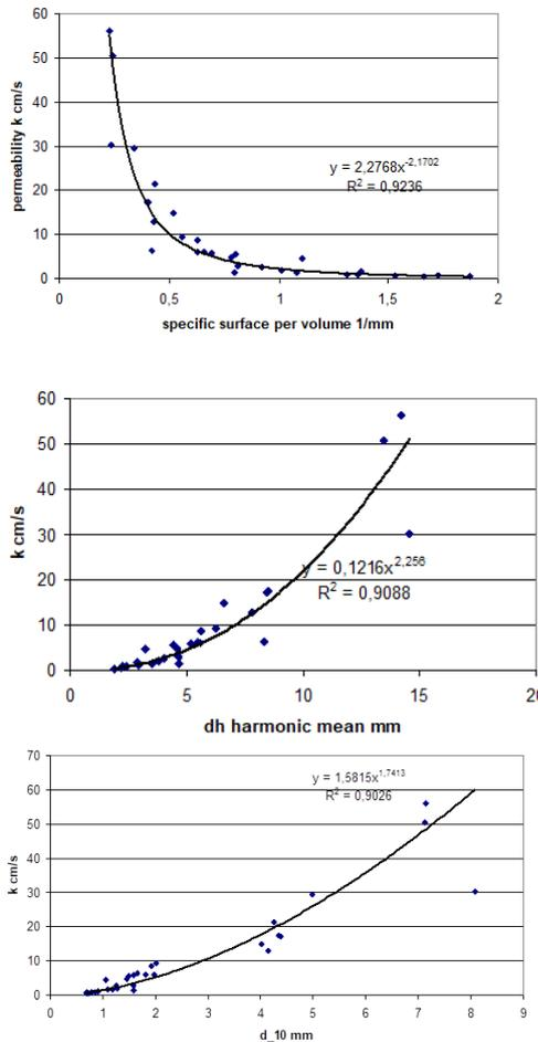
**Figure 18.** Re-evaluation of data of Feng in terms of various diameter values (specific surface parameter (containing density info), harmonic mean  $d_h$  and  $d_{10}$  with  $R^2=0.92, 0.91$  and  $0.90$  resp.).
