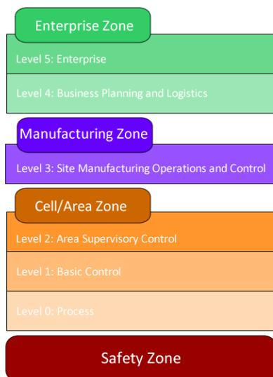
Figure 2.1 Purdue model for control hierarchy logical framework by SANS
