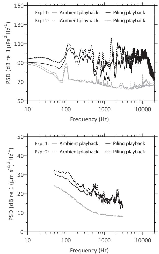
**Fig. 1.** Power spectral density of sound playback exposures. RMS power spectral density of received ambient- and piling playback in each experiment as recorded in exposure vessels. Top: sound pressure; 0.1 s Hann window and 50% overlap. Bottom: particle motion; 0.1 s Hamming window and 50% overlap.
