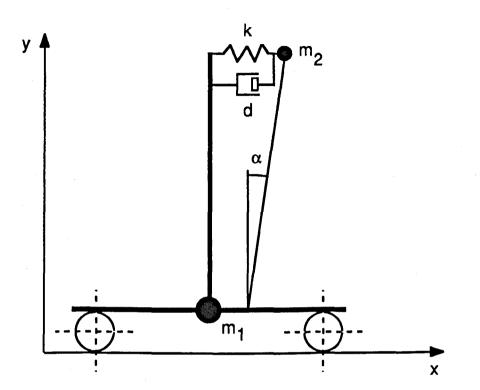
Fig. 3.1 Two mass equivalent model of a stacker crane
