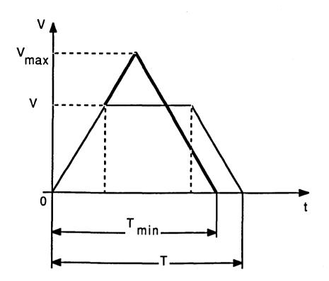
Fig. 3.2 Optimum velocity-time graph.
