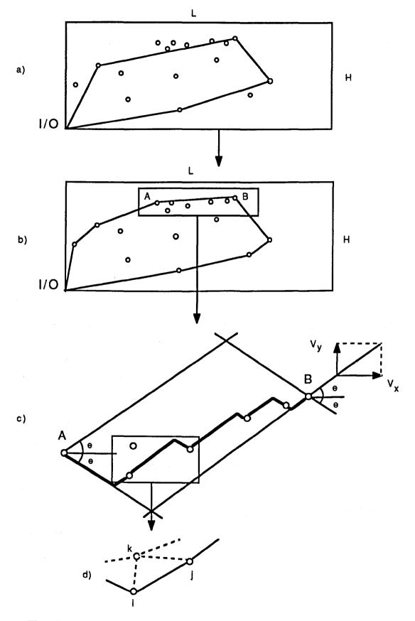
Fig. 3.4 Main steps of Chebhull algorithm
