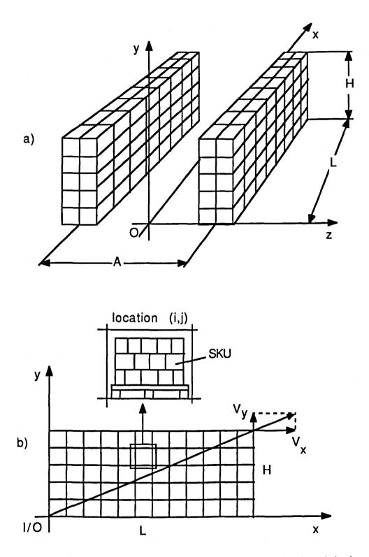
Fig.1.2 An aisle in a high bay warehouse; a) pictorial view; b) front view of a rack
