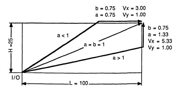
Fig. 3.7 Difference between rack shape factor and velocity vector
