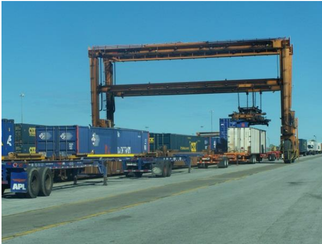
Figure 2. Crane unloading train onto chassis. (Source: authors)
