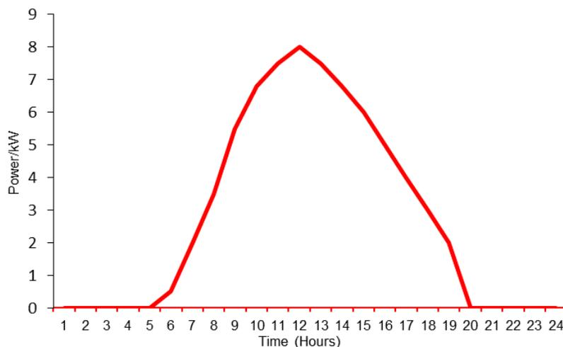
Figure 6. The generation profile of PV generators.
