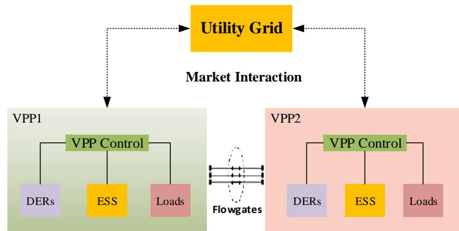
**Figure 2.** The structure of the interconnected VPPs with the utility grid.
