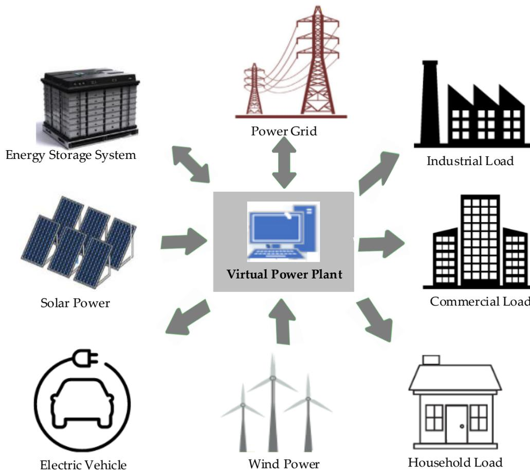
**Figure 1.** A generic structure of a virtual power plant.
