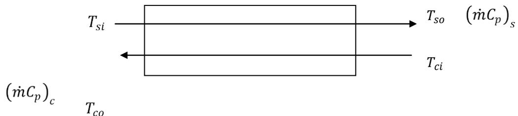
Figure 4. 5: Schematic of an adiabatic counter-flow heat exchanger (Duffie & William 2012).
