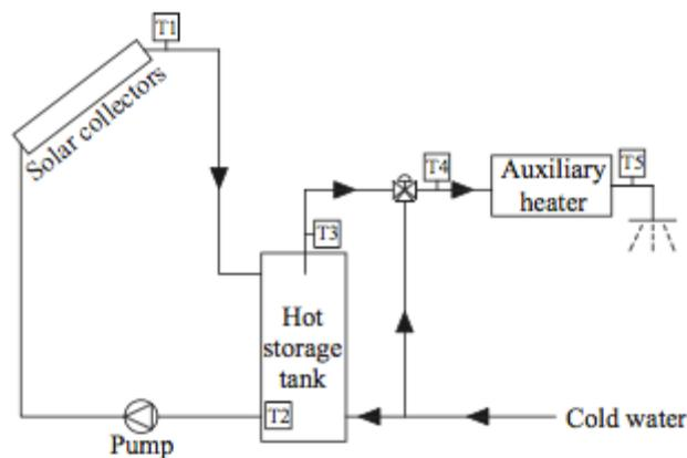
Figure 3.5: Schematic diagram of a solar water heating system Marken (2009).
