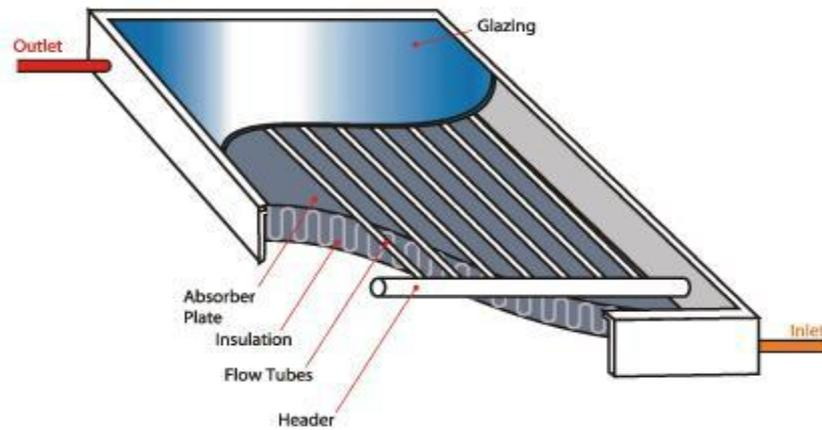
Figure 4. 4: Solar flat plate collector
