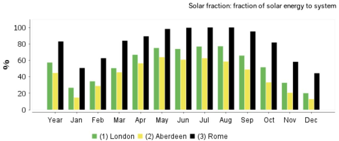
Figure 5. 12: Fraction of solar energy to system
