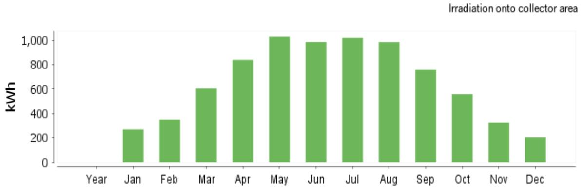
Figure 5. 2: Radiation into the solar collector
