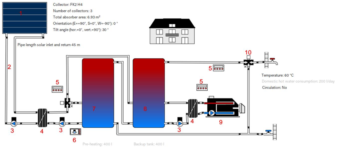
1 = Collector, 2 = Connecting pipes, 3 = Solar pump, 4 = Heat exchanger, 5 = Auxiliary heating control, 6 = Variable speed controller, 7= Pre-heating tank, 8= Backup tank, 9= Auxiliary boiler, 10= Mixing valve controller
