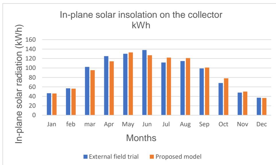
Figure 5. 15: In-plane solar radiation
