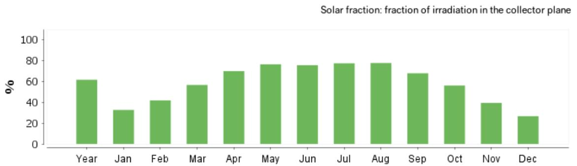
Figure 5. 3: Solar fraction of irradiation in the collector plane
