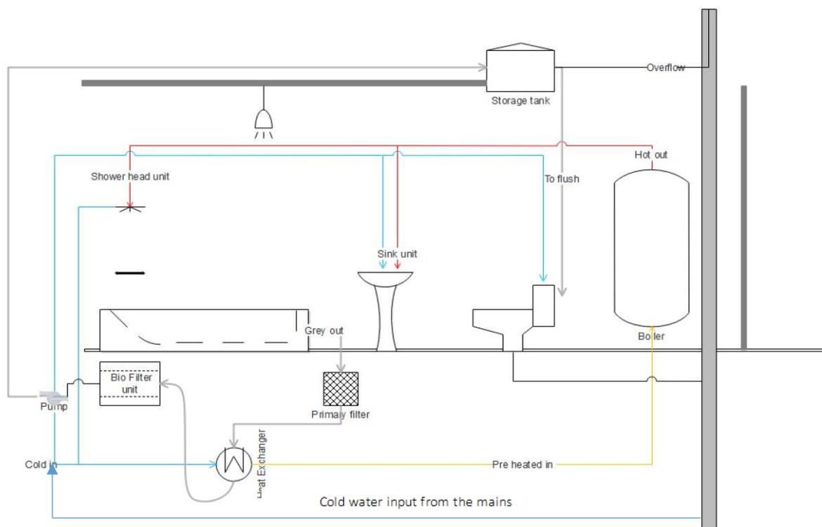
Colour codes: Blue – cold water input, yellow – preheated water, red – hot water
