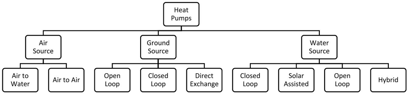
Fig. 9. Heat pump types.
