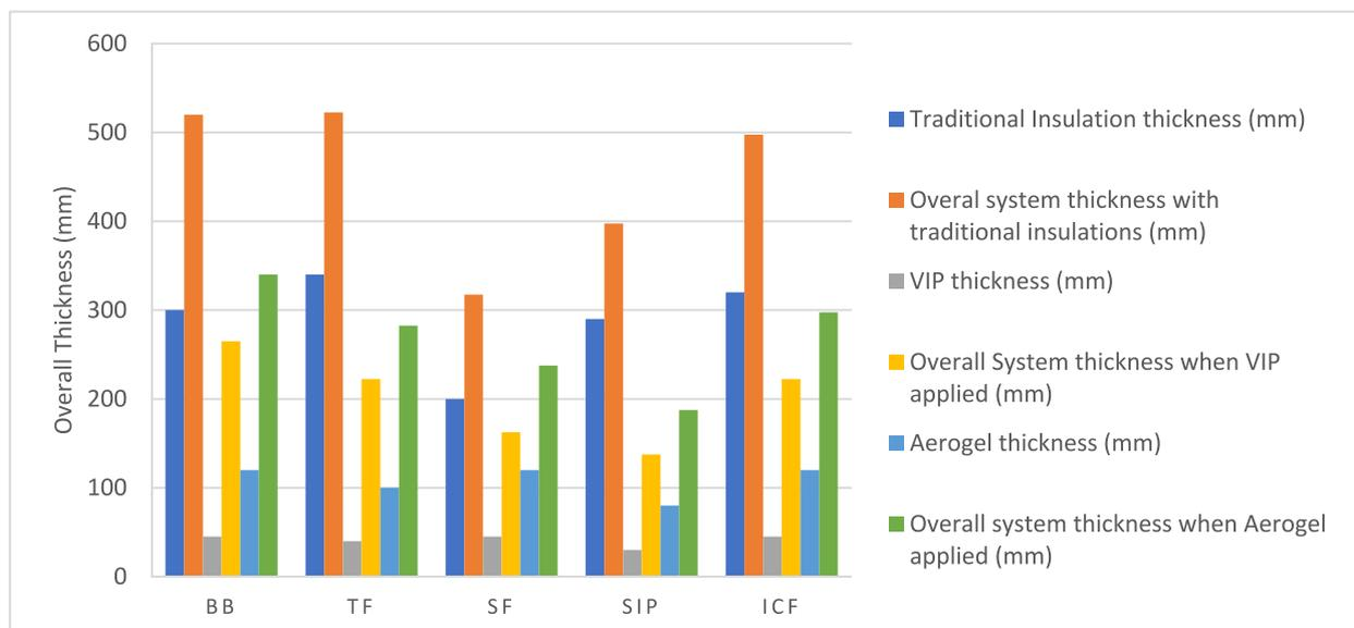
Fig. 7. Most common construction system in the UK when traditional (rockwool) and modern insulations applied to achieve 0.1 U-Value.
