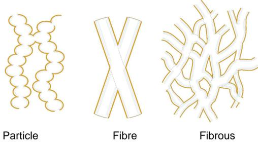
Cellulose comes in many different sizes and morphologies and is one of the most abundant biopolymers on earth. Its insolubility in water, low temperature pyrolysis and low cost makes it an excellent candidate to use as a pore former in the manufacture of SOFC electrodes via Electroless Co-Deposition [6].
