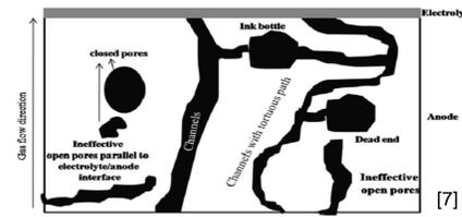
An interconnected pore network will provide greater opportunity for the fuel gas and resultant waste gases to diffuse in (and out) as well as increasing the triple phase boundaries within the electrode, producing a SOFC with a higher power density [1].
