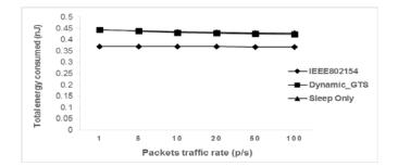
Fig. 10. Total energy consumed for an increasing packets rate
