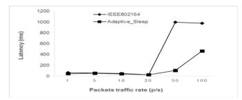
Fig. 3. End-to-end delay for an increasing packets rate
