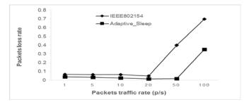
Fig. 2. Packets loss for an increasing packets rate
