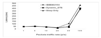
Fig. 12. End-to-end delay for an increasing packets rate
