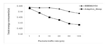
Fig. 7. Total energy consumed for an increasing packets rate
