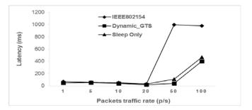
Fig. 9. End to end delay for an increasing packets rate
