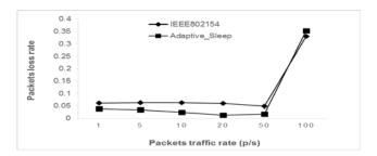
Fig. 5. Packets loss for an increasing packets rate
